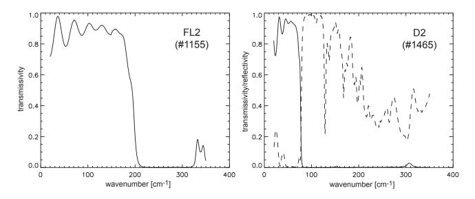
Figure 2. Typical filter curves of filters used in FIFI LS (compare Table 1). Left: Transmissivity of filter FL2. Right: Transmissivity and reflectivity of dichroic D2. Transmissivities are shown in solid lines, reflectivities in dashed lines.
