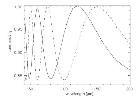
Figure 3. Transmission curves for 40  $\mu$ m (solid line) and 50  $\mu$ m (dashed line) polypropylene foil used as window material for FIFI LS.
