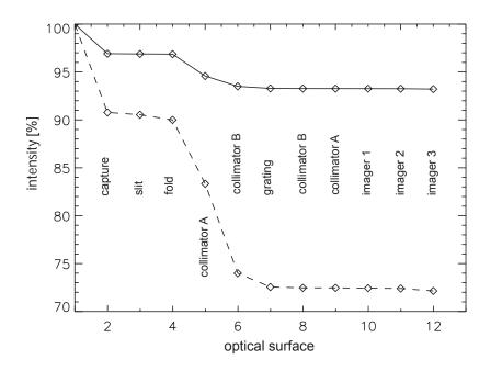
Figure 8. The light loss through the long wavelength spectrometer (for 160  $\mu$ m) due to diffraction effects and vignetting by the indicated optical surface. The solid line shows the light loss through the central slice, the dashed line through the first off-center slice respectively.
