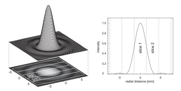
Figure 7. The image of a monochromatic (160  $\mu$ m) point source at the slicer mirrors of FIFI LS. Left: Three dimensional representation of the diffraction pattern (Airy function) and the projected intensity. The white rectangles represent the individual slicer mirrors and show how the mirrors cut into the Airy disc. Right: The intensity as a function of radial distance. The dotted vertical lines indicate the width of the individual slicer mirrors.
