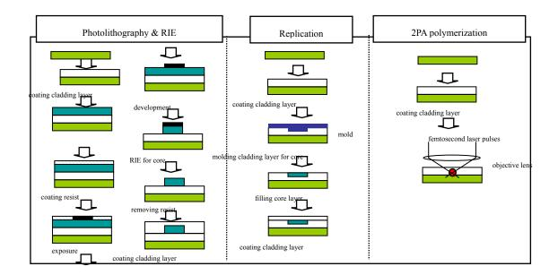
Figure 2 Optical waveguide fabrication methods
