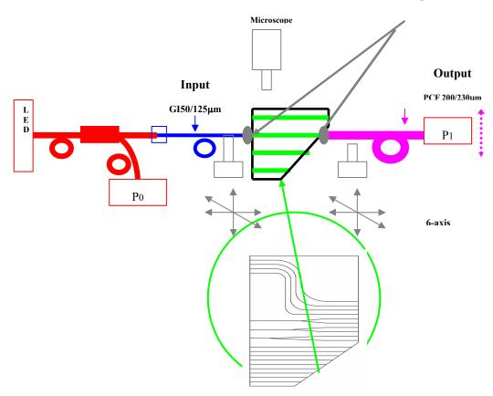
Figure 8 Measurement set-up for optical waveguide chip
