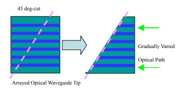
Figure 5. Fabrication of waveguide for loss measurement.
