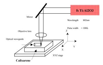
Figure 3 Experimental set-up of TPAP method
