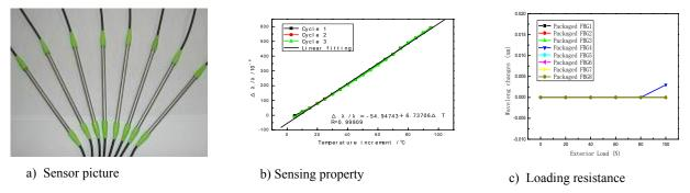
Figure 3. Novel FBG temperature sensors without exterior load influence
