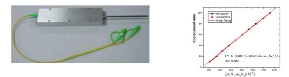
Figure 6. FBG displacement transducer developed at HIT
