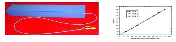
Figure 7. Novel ice load cell based on dual FBGs
