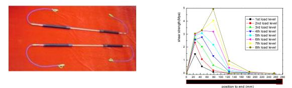
Figure 14. Smart FRP anchor based on FBG
