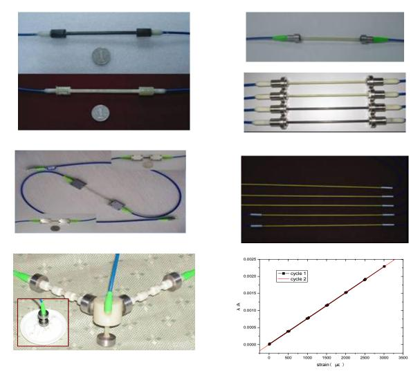
Figure 1. Various FRP-Packaged FBG strain sensors
