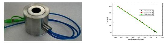
Figure 8. Novel ice load cell based on dual FBGs
