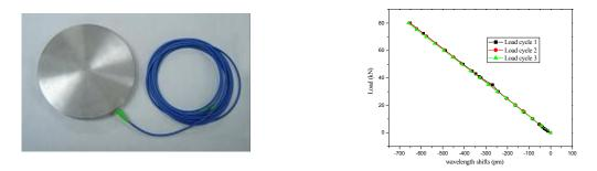
Figure 11. Novel ice load cell based on dual FBGs
