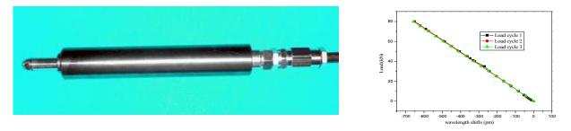
Figure 10. Novel ice load cell based on dual FBGs
