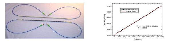
Figure 12. FRP-OFBG rebars and their sensing properties
