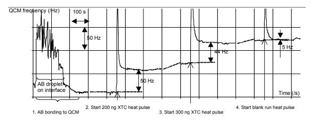
Figure 12. Measured system response to the subsequent loading of the system with 1) antibodies, 2) 200 ng ecstasy vapour, 3) 300 ng ecstasy vapour and 4) a blank run. The extreme pressure sensitivity of the QCM can be observed during the fluidic stabilisation of the interface after droplet addition (step 1), whereas the extreme temperature sensitivity shows in the direct response to the heat pulse (step 4).
