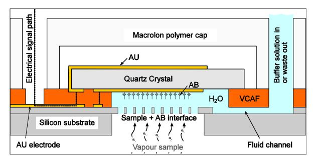
Figure 8. Schematic cross-sectional view of the four-component system.
