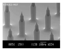
Figure 2: SEM picture of several microneedles. The length of the needles is 400  $\mu$ m. Each microneedle chip contains 25 needles.
