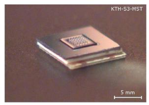
Figure 4: Picture of an assembled drug delivery unit. The device can store  $12 \ \mu$ l of liquid.
