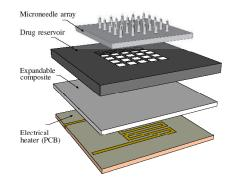
Figure 3: Exploded view of the microfabricated drug delivery system.
