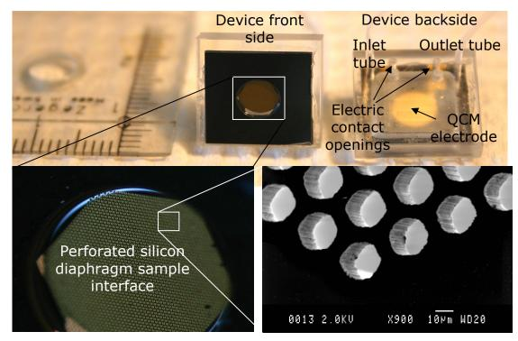
Figure 9. Front and backside picture of two devices. The QCM crystal is visible through the macrolon backside cover cap. The SEM insert shows the 20 µm thick diaphragm with hexagon shaped 25 µm diameter holes with wall thickness of 10 µm.
