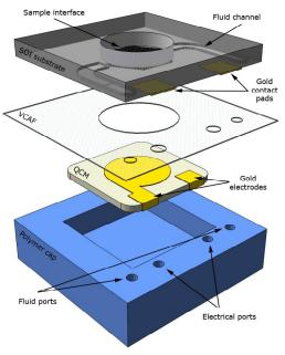
Figure 10. Exploded schematic of the four-component system
