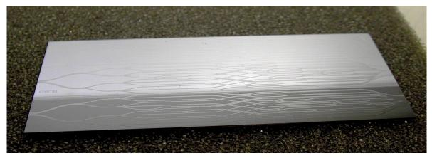
Figure 11: Integrated optics beam combiner prototype
