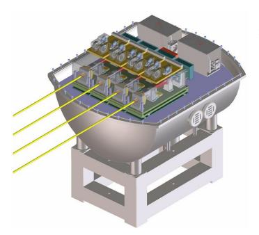
Figure 9: The GRAVITY beam combiner instrument.
