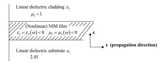
Fig. 7. A nonlinear slab of negative index material [NIM]
