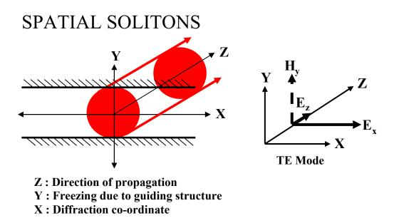
Fig. 1. A sketch of how a spatial soliton can be formed within a planar waveguide. The propagating mode is an envelope that is quasi-TE
