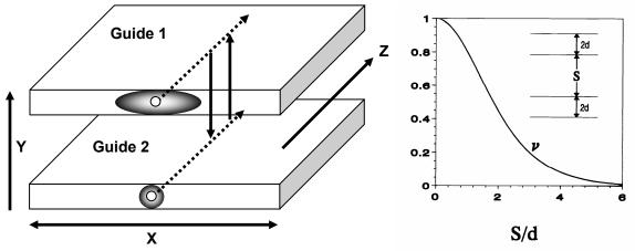
Fig. 5. Sketch of a planar waveguide structure. Guide 1 is made of a normal positive phase medium. Guide 2 is diffraction managed. The graph showing  $\nu$  sketches the extent of linear coupling as a function of guide separation.
