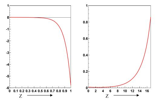
Fig. 8. The field profile across the film for (a) an order 1 solution and (b) an order 0 solution respectively.
