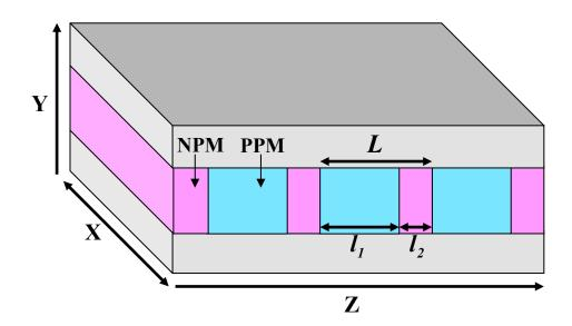
Fig. 2. A diffraction-managed waveguide. PPM is a positive phase medium, and NPM is a negative phase medium.
