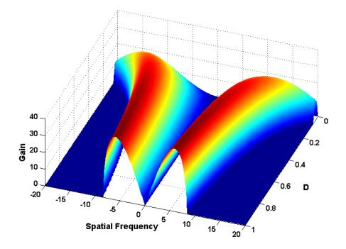
Fig. 3. Regions of gain for a range of diffraction management parameters against transverse wave number.  $\kappa = 0.0018$  and  $P_0 = 20$ .
