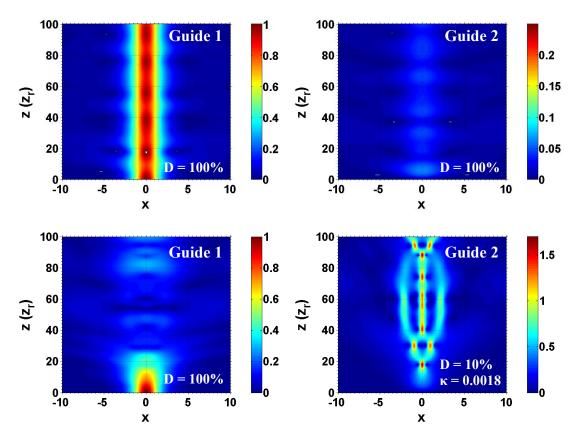
Fig. 6. The coupling between a pair of waveguides is shown for two cases. For the upper set D = 100% in both waveguides, and the small linear co-efficient  $\nu = 0.1$  prevents a transfer of energy. In the lower set, both diffraction management and nonlinear diffraction facilitates a strong energy transfer. The initial input in both cases is  $\psi(x, 0) = sech(x)$  to guide 1.
