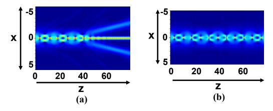
Fig. 4. Generic pictures of soliton formation for D =10 %. Z is the direction of propagation and is measured in Rayleigh lengths, and X is the diffraction direction, and is measured in beam widths. (a) In the absence of nonlinear diffraction an initial  $\psi(x, 0) = sech(x)$  input yields a low order breather. (b) Addition of nonlinear diffraction causes breather to break up. D = 10% including nonlinear diffraction with  $\kappa = 0.0018$ .
