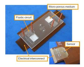
Figure 3: Microfluidic and electrical interconnect functions integrated into a lab-on-chip device.
