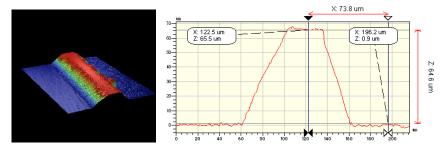
Figure 4: Visualization and dimensional measurement of the knife-edge used for gluing.
