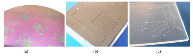
Figure 7: Microfluidic structure embossed into plastic using an epoxy mold insert
