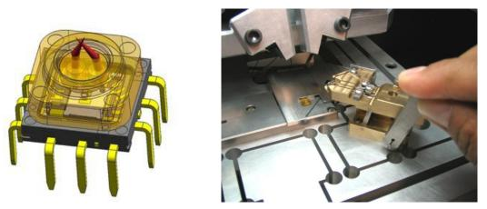
Figure 11: Philips Twin - Eye Laser Sensor - product and tester
