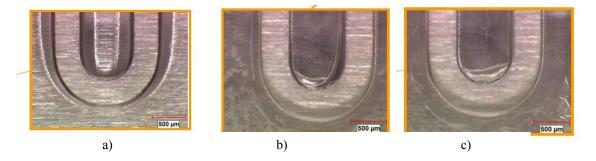
Figure 8: replication of a section of a serpentine-like microfluidic channel via hot-embossing at different mold temperatures: a) 140 °C, b) 190 °C, c) 220 °C
