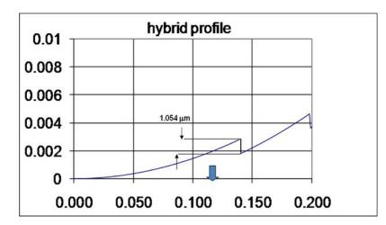
Figure 1: theoretical profile of a diffractive element superimposed upon an aspheric surface
