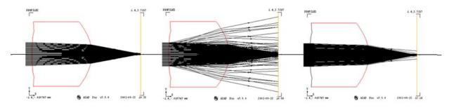
Figure 2: simulation of lens performance with ideal profile, large draft angle, optimized draft angle
