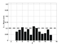
Figure 18. Aberration reproducibility versus Zernike number at the Zeiss actinic metrology test stand. Dotted line represents the requirement.
