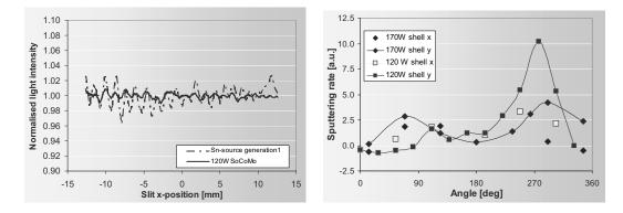
Figure 4. Left: champion data of slit uniformity with the first generation Sn source and the 120W source. Right: comparison of the angular dependence of the collector sputter rate in 120W and 170W source configurations for two shells x and y.
