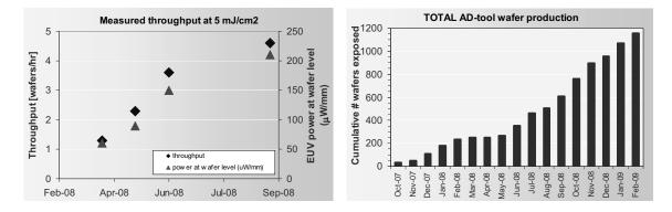
Figure 3. Left: measured throughput and power at wafer level *versus* time in one of the ADTs with a 120W source. Right: cumulative amount of wafers exposed in the ADTs - close to 1200 300-mm wafers for R&D were exposed so far.
