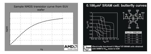
Figure 13. Left: electrically functioning transistor of which the first metal level was exposed on  $ADT^{[1]}$ . Right: electrically functional 0.186  $\mu m^2$  6T-SRAM cell, of which the contact hole layer was exposed on  $ADT^{[3]}$ .
