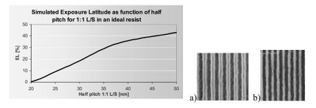
Figure 7. Left: Simulated exposure latitude as function of half pitch in an ideal resist. Right: a)  $28 \text{nm}^{[13]}$ ; and b)  $26 \text{nm}^{[15]}$  1:1 L/S imaging demonstrated on ADT.
