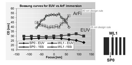
Figure 11. Bossungs curves for 28nm WL1 and SP0 with EUV (NA=0.25,  $\sigma$ =0.5) compared to 40nm WL1 and 60nm SP0 with ArF immersion (NA=1.35,  $\sigma$ =0.82/0.97 dipole-X with 35° opening angle, Y-polarized)..
