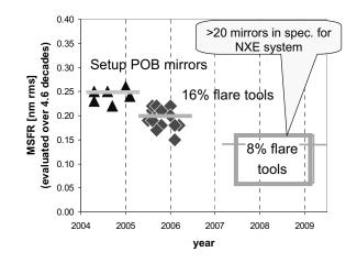
Figure 16. Progress in mirror polishing (MSFR), supporting <8% flare performance.
