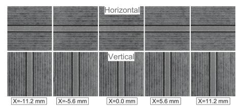
Figure 10. CD SEM pictures from the 28nm half pitch Flash modules across the exposure slit.
