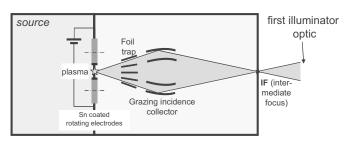
Figure 2. Schematic overview of the ADT Sn source.
