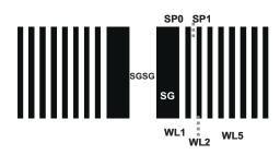
Figure 8. Schematic representation of the word line/gate layer and the features that are evaluated. Space SGSG is designed as 4x the word line half pitch, select transistor SG as 2.5x the word line half pitch, spaces SP0 and SP1 both have the word line half pitch, just like word lines 1, 2, and 5.
