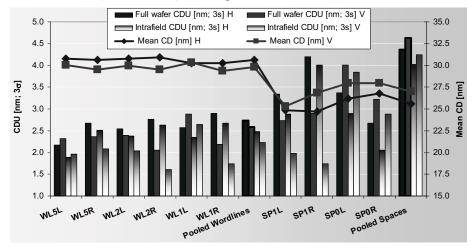
Figure 9. Mean CD, full wafer and intrafield CD uniformity for all evaluated word lines and spaces in the gate layer, both left (L) and right (R) of the central space (SGSG), for 28nm half pitch design rule. The pooled word lines meet the 2.9 nm CDU requirement in the ITRS.
