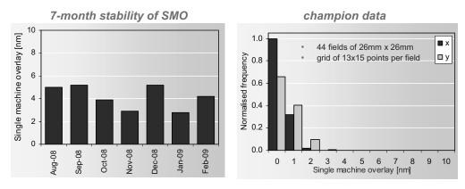
Figure 5. ADT single-machine overlay stability (left) and histogram of champion data (right).
