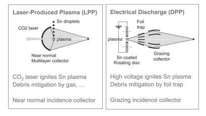
Figure 19. Key elements of sources for high volume manufacturing: LPP (left) and DPP (right).
