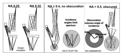
Figure 15. Possible optics design roadmap down to 11nm resolution with >0.4NA optics. All four diagrams are design examples.
