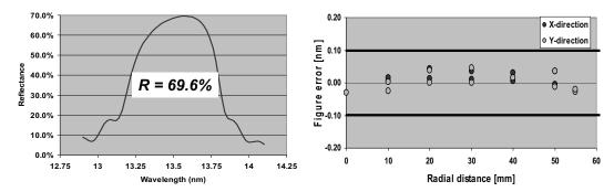
Figure 17. Left: mirror coating development for NXE has yielded >69% peak reflectivity. Right: added figure error due to the coating process for various lateral positions on the mirror.
