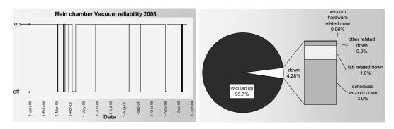
Figure 6. Vacuum reliability of the ADTs is high; the uptime of the main chamber (including optics and stages) exceeds 95%, measured over a 49-week period (total: 8232 hrs).
