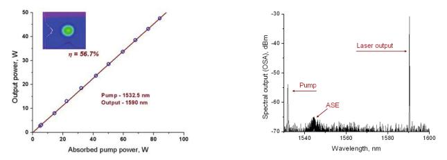
**Figure 2.** Output versus absorbed pump power dependence obtained for the resonantly cladding-pumped Er-doped FBG-laser shown in Fig.1.
