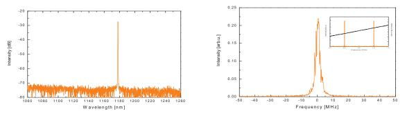
Fig. 2 Spectrum of the amplifier output. left) a broad range spectrum taken with an Ando spectral analyzer showing 40 dB contrast; right) a detailed spectrum of the 3.5MHz line taken with a Fabry-Perot interferometer (1 GHz FSR).
