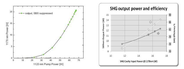
Fig. 1 Left: output power of the 1178nm fiber Raman amplifier as a function of pump power;Right: measured SHG output power at 589nm, up to 14.1W CW in this plot, with conversion efficiency up to 82%
