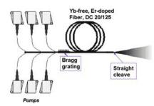
**Figure. 1.** Optical layout of the resonantly cladding-pumped fiber laser based on Liekki Er60-20/125 DC fiber pumped at 1532.5 nm.
