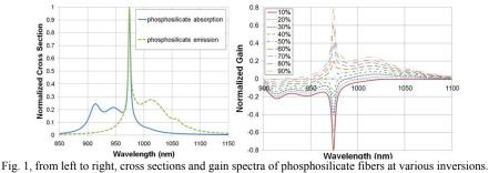
We demonstrate in this work phosphosilicate fibers fabricated with an optimized CVD process for high phosphorus and rare earth doping. Ytterbium-doped fibers are demonstrated to have phosphate-like spectral
