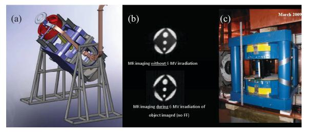
Figure 2. The Edmonton MR-linac design. (a) A rotational assembly carries a permanent magnet (blue) that rotates with respect to the patient. The accelerator is mounted orthogonal to the rotational axis and also rotates about the patient. (b) An MR image of a test phantom acquired with and without the radiation beam operating. (c) A photo of the current, non-rotating assembly. Figures provided courtesy of Gino Fallone.
