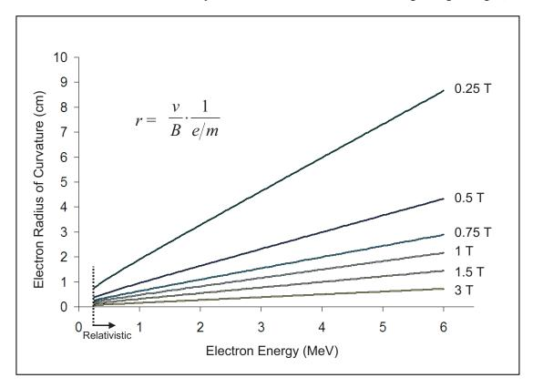
Figure 4. Relationship between the radius of curvature and the kinetic energy of an electron travelling orthogonal to the magnetic field. For relativistic energies, the dependence on electron energy appears linear. This has been plotted for a range of magnetic field strengths being considered for MRgRT systems. The range of electron energies is large corresponding to the continuum of electron energies produced in Compton scattering events and the polyenergetic spectrum of a 6MV photon beam.
