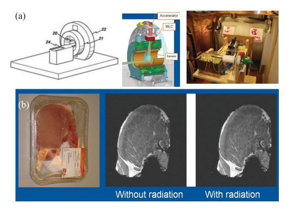
Figure 1. The Utrecht MR-linac design. (a) A key development is the modification of the magnet to create a low-field envelope around the magnet in which the electron gun and transport mechanism can operate, regardless of angle. (b) An image of butcher's meat acquired at 1.5T without and with irradiation by the 6MV photon beam. Figures provided courtesy of Jan Lagendijk.
