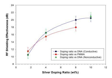
Figure 4. RF shielding effectiveness versus Ag doping ratio for both DNA-CTMA+Ag and PMMA+Ag.
