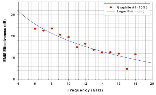
Figure 6. EMI effectiveness versus frequency for 10 wt% graphite filler in DNA-CTMA
