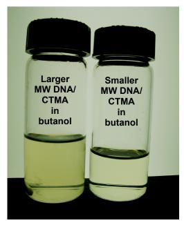
Figure 1. Comparison of DNA-CTMA solutions made using larger and smaller MW DNA.
