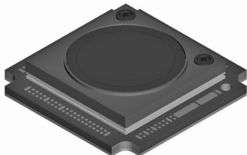
Fig. 17 Compact room-temperature avalanche-photodiode package containing a 256 \times 256 HgCdTe array with a readout that can process multiple signal returns from a pulsed laser.
