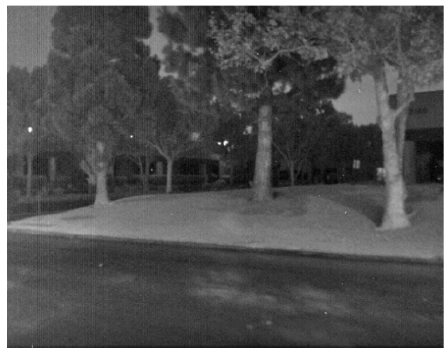
Fig. 9 A SWIR image taken with a 640 \times 480 InGaAs array under minimal street-lighting conditions.
