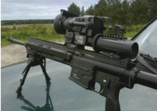
Fig. 2 Carl Zeiss Optronics' IRV 900 mounted on an HK 417 rifle in front of a 4×30 day-sight aiming optics.
