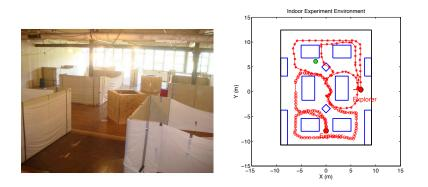
(a) Picture of the indoor environment (b) Schemetic of the indoor experiment environment for mapping
