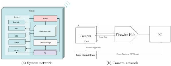
Figure 3. Network scheme and camera interface design
