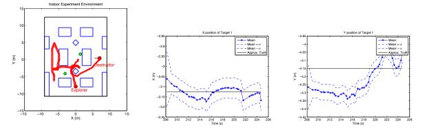
(a) Schematic of the indoor experi- (b) Mean and Covariance for target 1 (c) Mean and Covariance for target 1 ment environment for neutralization in X-direction in Y-direction process
