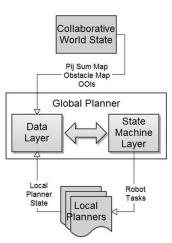
Figure 10. The two tiered planning system separates task allocation from path planning and following
