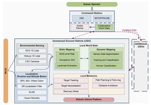
Figure 1. System architecture for Cornell's distributed human-robotic testbed.
