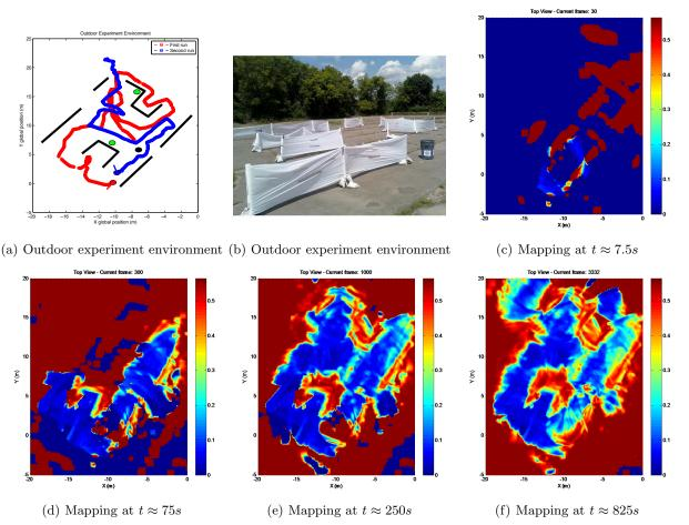
Figure 15. Outdoor experiment environment schematic and pictures including robots' trajectory. Mapping results are shown at four different times.
