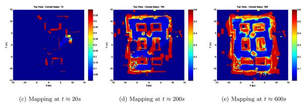
Figure 13. A picture(a) and a schematic(b) of the indoor environment with mapping results. Red circles denote two robots' initial positions and heading, and green circles represent targets. A path with circles and a star is drawn for each robot. The bottom figures (c - e) show an overhead-view map generated by two robots at three different moments.
