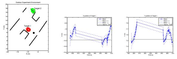
(a) Outdoor tracking showing covari- (b) Mean and covariance for target 1 (c) Mean and covariance for target 1 ance circles for two targets in X-direction in Y-direction
