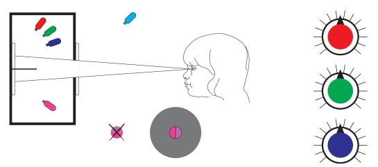
Figure 7. Elements and steps of the color matching experiments. The three knobs at right are turned until the two halves of the bipartite field match. If a match cannot be achieved, a primary source is moved to the other side to desaturate the test color; the corresponding knob is given a minus sign. The optional light source outside the box can be used to create a surround for adaptation.
