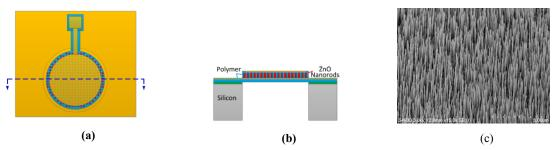
Figure 10. (a) Top-view and (b) cross-section view of the acoustic sensors designed with polymer matrix piezoelectric nanocomposites. (c) SEM images of vertically aligned ZnO nanowires grown on a sapphire substrate.
