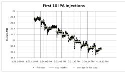
Figure 3. Full data collection run recorded with a tin oxide sensor and the wireless system
