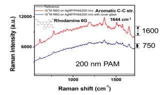
Figure 4. Raman response with and without pyrex cover for Rhodamine6G.
