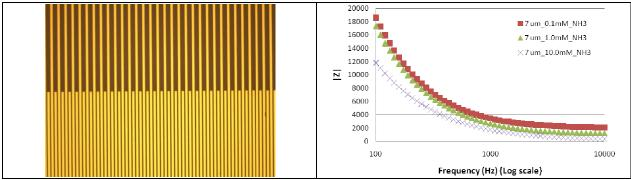
Figure 8. a) 7 µm Gap Electrodes. b) Total Impedance vs. Frequency for the 7 µm Gap Electrodes.
