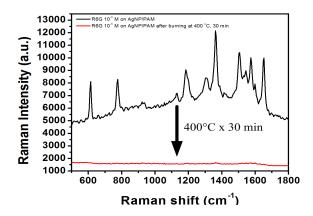
Figure 6. Silver NP based SERS are not compatible with anodic bonding in the presence of oxygen gas
