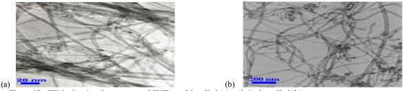
Figure 13. SEMs showing the structure of CNTs, multi-walled (a) and single-walled (b).
