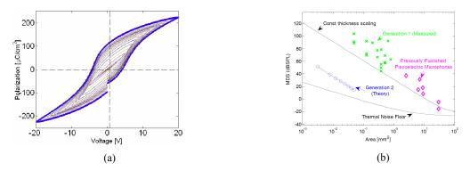
Figure 12. (a) Measured hysteresis loops of polarization versus applied voltage. (b) The measured MDS data of the Generation 1 sensors and the predicted values of the Generation 2 sensors as compared to previously published piezoelectric acoustic sensors reported in the literature<sup>13-18</sup>.
