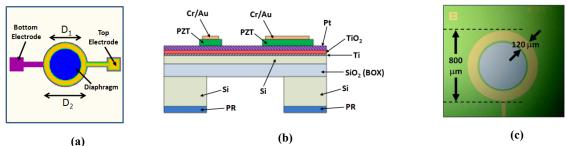
Figure 9. (a) The top view of the acoustic sensor showing the top and bottom electrodes and the diaphragm. (b) A crosssection of the sensor showing layer stack and the etched areas. (c) An optical micrograph of a fabricated acoustic sensor
