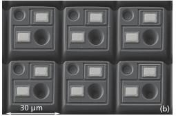
Fig. 13 Dual-band MWIR/MWIR Type II superlattice pixels with reduced  $-30 \ \mu m$  pixel size.
