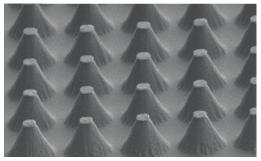
Fig. 18 Pyramidal absorbers on an InAsSb layer were structured to increase photon absorption.
