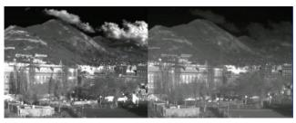
Fig. 25 Imagery taken with a dual-band MW/MW array of HgCdTe on CdZnTe having 24  $\mu$ m pitch in a 640 x 512 format.
