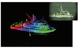
Fig. 21 3D image of a ship (visible insert) made with a scanned linear array of hole-avalanche HgCdTe detectors.
