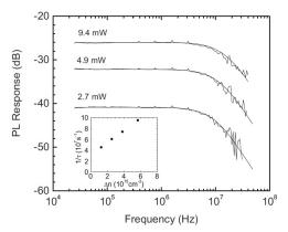
Fig. 14 Photoluminescence-decay measurements made on an LWIR Type II superlattice sample showing a lifetime of 31 nsec for the low-flux limit of photo-excitation.
