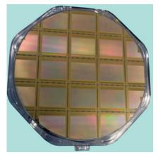
Fig. 6. 2048 x 1536 uncooled VO<sub>x</sub> microbolometers with 17  $\mu$ m pixel pitch on a 200 mm wafer.
