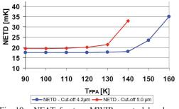
Fig. 19 NE $\Delta$ T for two MWIR spectral bands noted—as a function of operating temperature.
