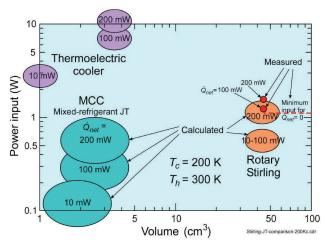
Fig. 30 MCC compared with thermoelectric and Stirling coolers for temperatures down to 200 K.
