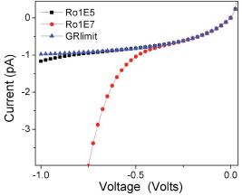
Fig. 29 Illustration of the impact of dislocation density on the reverse-bias characteristics of a HgCdTe diode.
