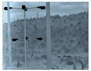
Fig. 17 Image taken at 150 K with an nBn  $640 \times 512$  array showing an NE $\Delta$ T of 20 mK. The dark spots on the hill are cows.
