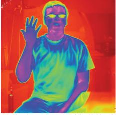
Fig. 12 Image taken with a 1K x 1K Type II superlattice FPA.
