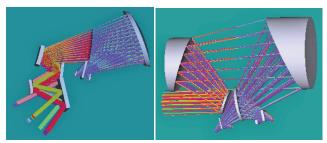
Fig. 2. Multi-band optical designs using three powered optical mirrors. The systems have two (left) and four (right) FPAs.
