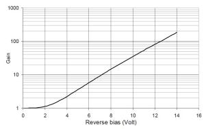
Fig. 20 Gain as a function of bias for a HgCdTe e-APD having a spectral cutoff of  $3.1 \,\mu\text{m}$  at 200 K.
