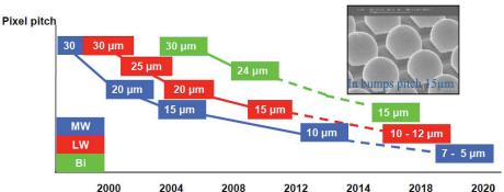
pulsing effects providing sub- Fig. 24 Progress (solid line) and projections (dashed line) for reducing pixel size for MWIR nanosecond time resolution. (blue), LWIR (red), and dual-band FPA applications.
