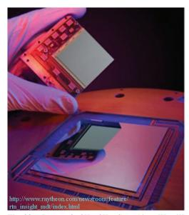
Fig. 23 Image of a 2K x 2K reflected in a 4K x 4K MWIR HgCdTe array grown on silicon.
