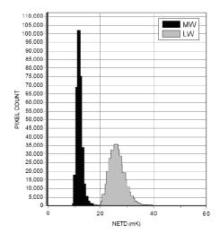
Fig. 26 Histograms of MW and LW band NE $\Delta$ T measured on a HgCdTe-on-GaAs array with 20  $\mu$ m pixels.
