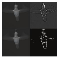
Fig. 5 The difference of Gaussian response of a hummingbird shows enhanced edge contrast as shown in the upper-right panel (input scene is in the upper-left). The zero-crossing image as shown in the lower-right image preserves the essential geometries in the scene, but conveys the information in a 1-bit representation. (Infrared imagery courtesy of the SE-IR Corporation, Goleta, CA)
