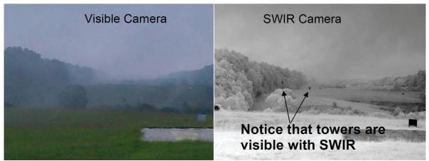
Fig. 15 Comparison of visible and SWIR imagery in atmospheric fog.
