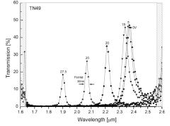
Fig. 16 Tuning range of a MEMs Fabry-Perot structure from 1.9 to 2.4  $\mu$ m with applied voltage noted above peaks.
