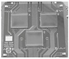
Fig. 9 The Thermal Infrared Sensor (TIRS) focal plane showing three QWIP sensor-chip assemblies.
