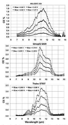
Fig. 10 Collection efficiency (CE) of QWIP FPAs from three NASA vendors as a function of wavelength for several bias values.
