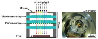
Fig. 3. (a) Compact multispectral camera integrated in cold shield. (b) Seen in opened laboratory dewar.
