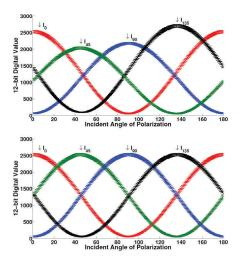
Figure 4. Average response of four polarization filter orientations before (top) and after (bot-tom) calibration.
