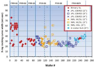
Fig. 11 X-ray crystal rocking curve data shows significant crystal quality improvement as experience is gained in growing Type II SLS material
