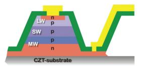
Fig. 28 Doping structure of a novel n-p-n dual-band HgCdTe pixel structure.
