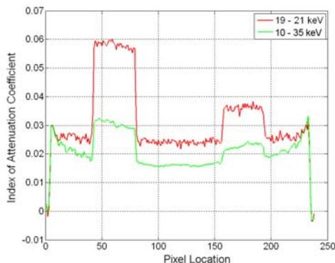
Figure 10 – The **green** profile is a CT value profile along a diameter of a plexiglas test phantom scanned with broad spectrum x-ray. It shows the cupping artifact due to beam hardening. The **red** profile is from the same diameter of the phantom, but from a CT image generated with the narrow bandwidth section selected from the broad spectrum scan data set. Note, the great reduction in beam hardening artifact and the increased noise (due to the fewer photons).
