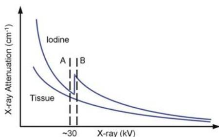
Figure 1 - A schematic representation of the change in x-ray attenuation coefficient with change in x-ray photon energy for iodine and for soft tissue. If x-ray images are generated from a narrow bandwidth x-ray spectrum, one just below and another just above the photon energy of iodine's K absorption edge, then their subtraction essentially removes the soft tissue but leaves a significant fraction of the iodine component of the image.
