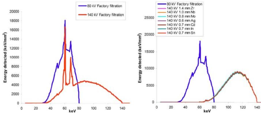
Figure 2 - *Left panel* shows a typical x-ray spectrum of a clinical CT scanner’s x-ray source operated at 80 and 140 kVp. These sources were both filtered with a layer of aluminum. Note the considerable overlap of the two spectra. The *right panel* shows the two spectra with the 140 kVp spectrum after filtration through various thin, fairly high atomic weight, metal foils. Reproduced with permission from Ref 3.
