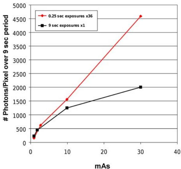
Figure 9 – The **black** curve indicates the impact of the heterogeneity of detector pixel saturation exposure as a function of total exposure. The **red** curve shows that if the same data are collected piecewise with a sequence of short-duration exposures, then the expected linear relationship results. See text for details.
