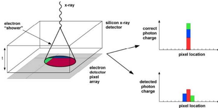
Figure 5 – *Left panel* is a schematic representation of the shower of electrons generated by the absorption of one x-ray photon. Note that this shower can affect the domain of several contiguous pixels. The *right lower panel* shows the charge recorded in each of those pixels. The *right upper panel* shows that one of the pixels is allocated one photon with an energy equal to the sum of the three, coincidentally recorded, signals.
