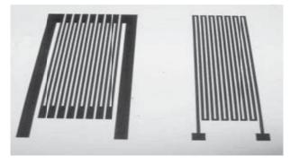
Figure 5. Printed strain gauge sensor.
