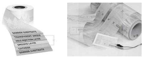
Figure 6. OLEDs devices printed on a flexible foil.
