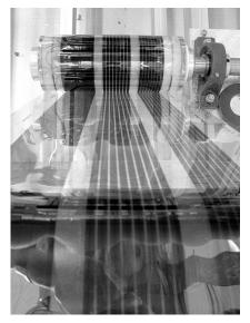
Figure 7. Organic Solar Cells printed on a flexible foil.
