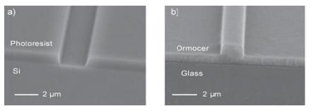
Figure 8. a) Imprinting mould consisting of patterned positive tone resist on a silicon wafer and (b) cross section image from a replicated ridge waveguide based on UV-curable hybrid polymer on a glass substrate.
