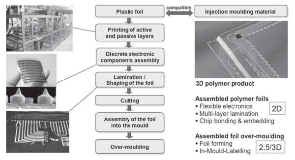
Figure 3. Printed Hybrid System concept utilizing plastic over-molding process.
