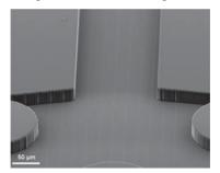
Figure 9. Waveguide structure combined with a microfluidic structure.
