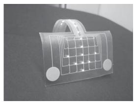
Figure 13. Display demonstrator with capacitive control switches.
