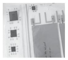
Figure 14. Flex-to-flex bonding test substrate containing secondary batteries and polyimide straps.
