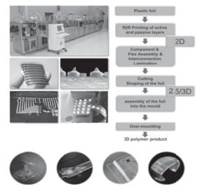
Figure 2. Printed Hybrid Systems concept is based on seamless combination of roll-to-roll printing, component assembly, lamination, foil forming and foil-over-molding processes.
