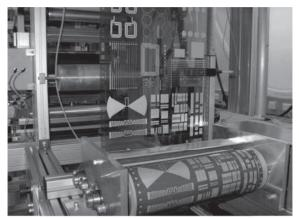
Figure 4. Roll to roll (R2R) printing machine producing printed electronics circuits.
