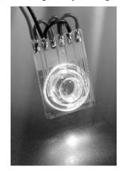
Figure 10. Over-molded illumination and imaging lens.
