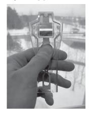
Figure 15. Over-molded OLED demonstrator.
