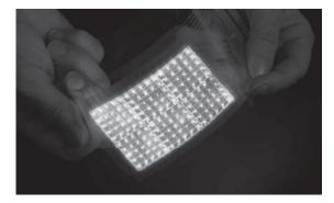
Figure 12. Assembled backplane with 6 x 25 laminated LED chips.
