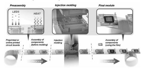
Figure 17. Stop and go roll-to-sheet production for Printed Hybrid Systems.
