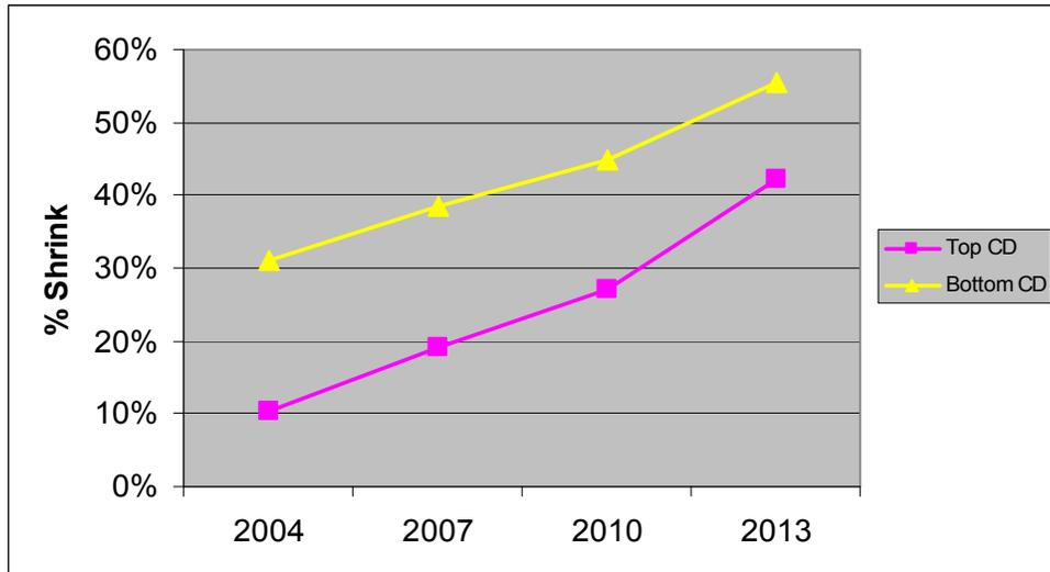
Figure 2. Contact CD Shrink Evolution for Immersion Lithography
