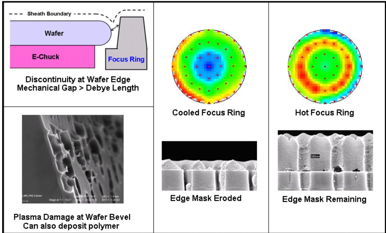
Figure 9. Discontinuity at wafer bevel
