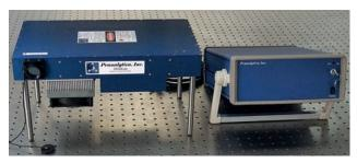
Figure 9. Photograph of the OmniLux laser system consisting four tunable QCLs covering a wavelength range from ~7 µm to 10 µm
