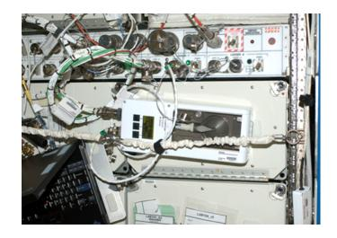
Figure 6. The Third Generation JPL ENose installed on EXPRESS Rack 2 on ISS.
