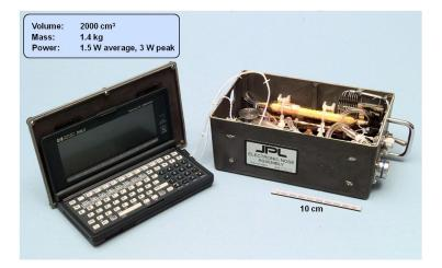
Figure 3. The First Generation JPL ENose flight unit. The palm top computer fit inside the container and was used for device control and data acquisition. This device had a volume of 2.0 liters, a mass of 1.4 kg and used 1.5 watts average power, 3 watts peak power.
