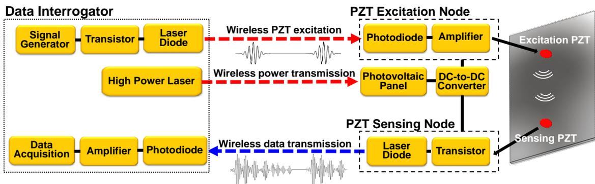
Figure 2. An overall schematic of the proposed optics-based wireless guided wave measurement system (—: wired electric connection, - ->: wireless laser)<sup>24</sup>
