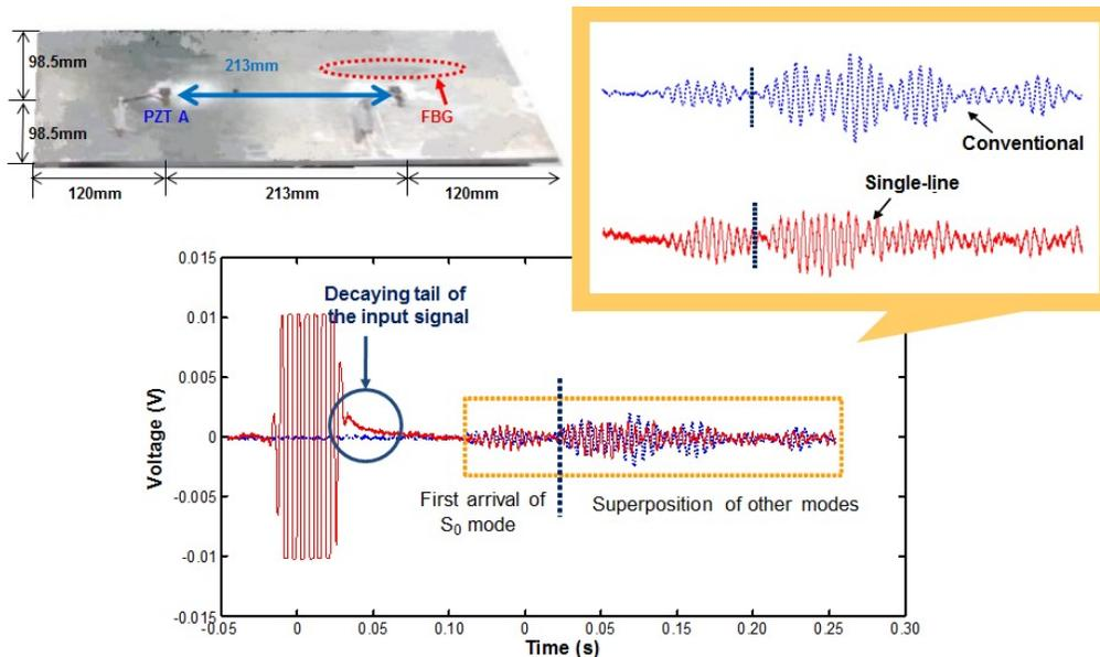
Figure 11. Comparison of ultrasonic signals obtained by the proposed PZT/FBG hybrid system (solid line) and the conventional measurement system (dotted line)
