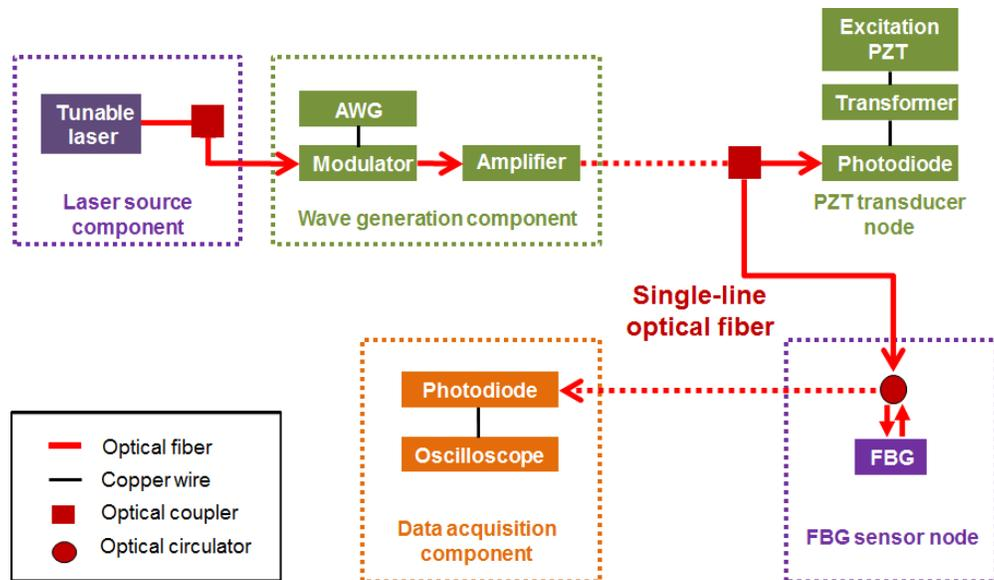
Figure 10. Integrated guided wave generation and sensing using a single laser source and optical fiber
