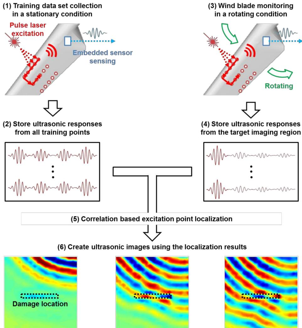
Figure 6. Overall scheme of the proposed laser ultrasonic imaging technique for a rotating blade. To collect training data, in Steps (1) and (2), ultrasonic waves are obtained by generating ultrasonic waves using a pulse laser excitation and measuring response using the embedded sensor, covering the entire training area by scanning the laser beam. In the wind blade
