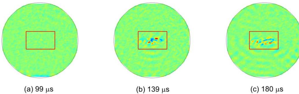
Figure 5. Isolating the standing wave components from the velocity fields in Figure 4
