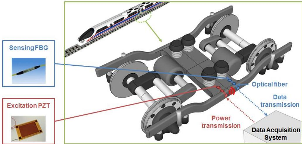
Figure 9. Monitoring of high-speed train bogie using embedded hybrid sensors and laser power/data transmission
