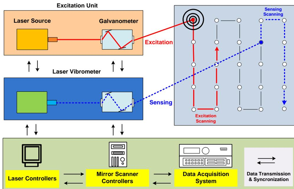
Figure 1. An overall schematic of the complete noncontact laser ultrasonic scanning system becomes of a Nd:Yag pulse laser, a laser Doppler vibrometer, scanning mirrors, and a controller.
