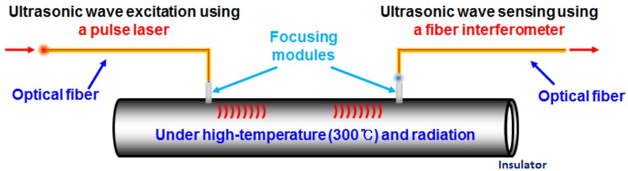
Figure 12. An optical-fiber guided ultrasonic excitation and sensing system for high temperature and radioactive environments
