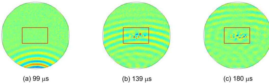
Figure 4. LDV imaging of Lamb wave propagation in a 1.8 mm thick graphite plate containing delamination. Standing waves are observed at the delamination site.
