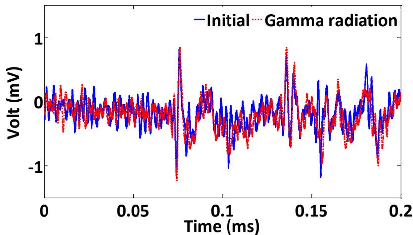
Figure 13. Comparison of ultrasonic signals obtained before (blue solid line) and after (red dotted line) exposing optical fibers to a typical 5 year Gamma ray radiation of 62.5 kGy
