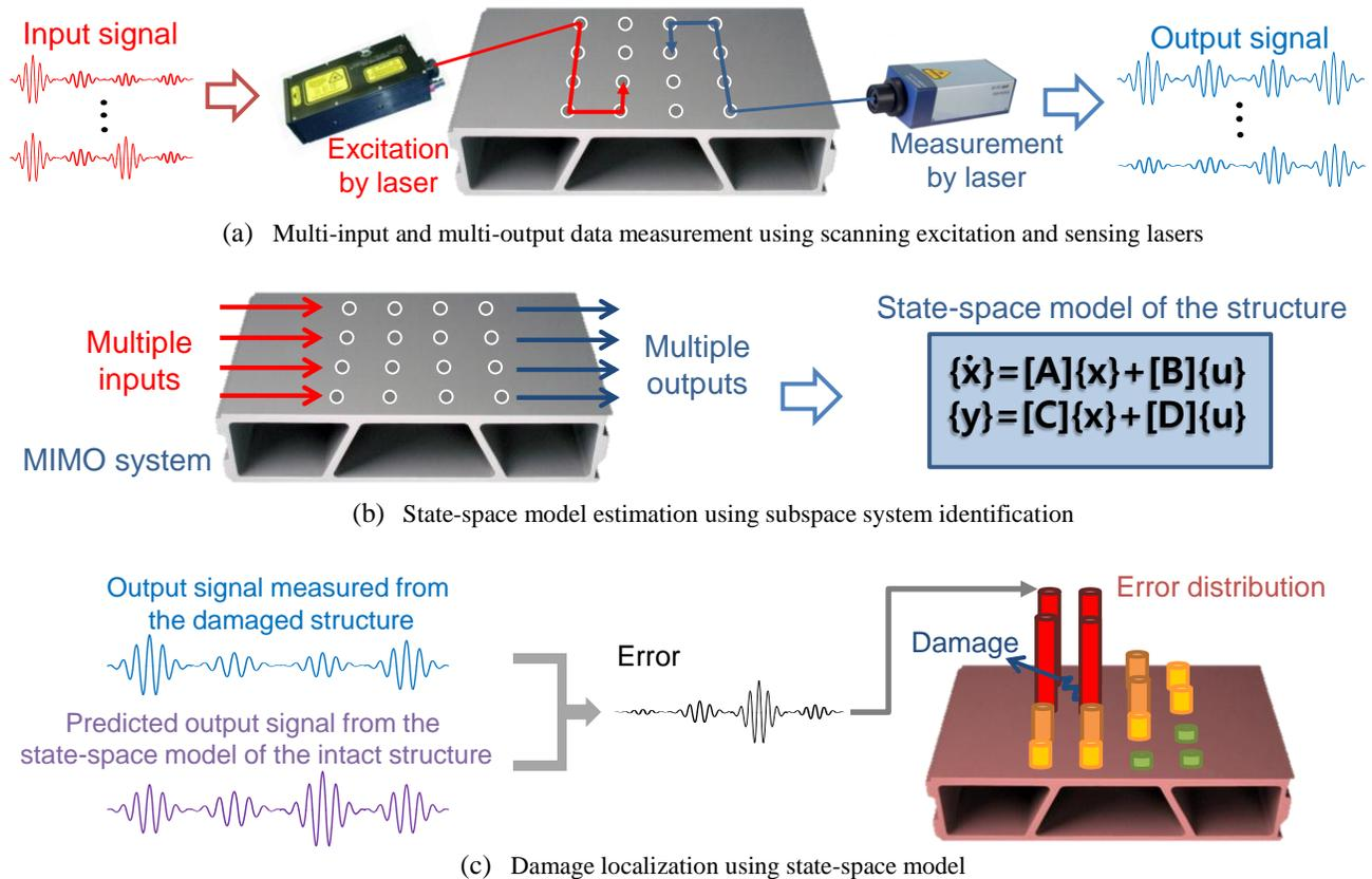
Figure 8. Local ultrasonic system identification for low-resolution estimation of a damage area
