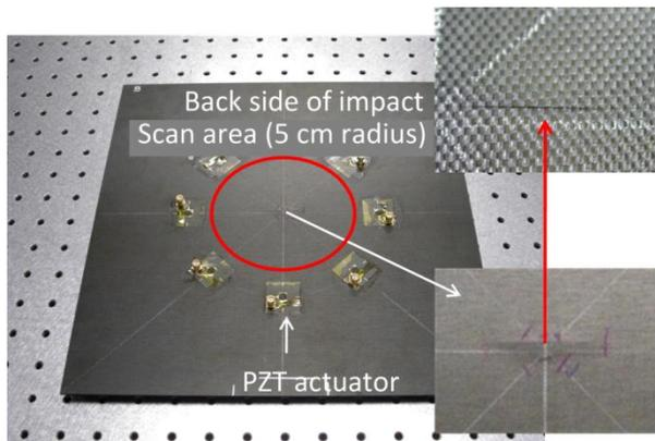
Figure 3. A multi-layer composite plate with impact-induced delamination
