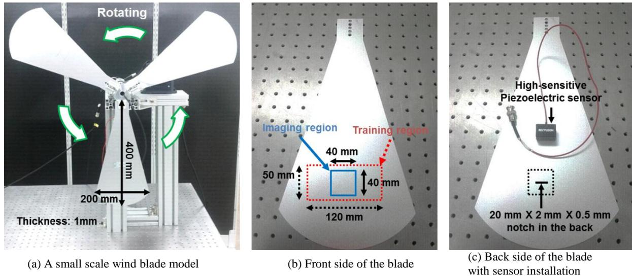
Figure 7. An aluminum wind blade model with a piezoelectric sensor installed at the back side of the blade. The black dotted box and the black solid box in (b) indicates the training region and the imaging region, respectively.
