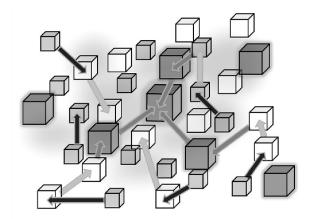
Figure 4. Scheme for an optical nanofountain comprised of 2-10 nm CuCl quantum dots, distributed in an NaCl matrix. The variation in size of different quantum dots brings into effect a spectroscopic gradient directed towards the largest units. Adapted from ref. 9.
