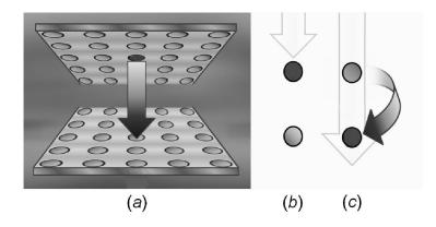
Figure 7. Depiction of a two-dimensional square-lattice configuration for an all-optical switching device: (*a*) side-view (not showing spacer layer between the two arrays); the initial excitation (dark grey dot) is transferred only to its partner directly underneath: (*b*) with the passive beam yet to enter there is no transfer of excitation, (*c*) with the beam passing though the system transfer does occur.
