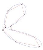
Figure 1. A contour C is sampled at N = 11 points, indicated with "X", and the samples connected to form a polygonal approximation.
