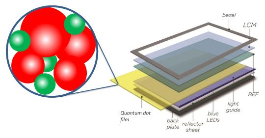
Figure 2: Schematic structure of an edge-lit LCD display with quantum dot film.
