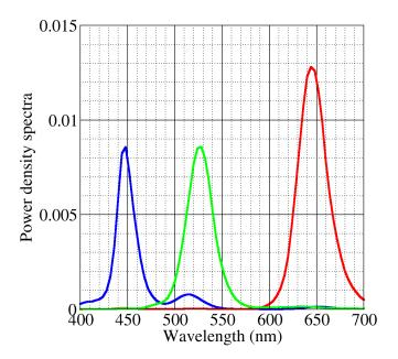
Figure 3: Power density spectra of the 3 primary colors from a demo LCD using QDEF for Rec. 2020 color gamut.
