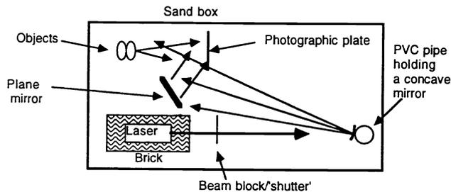
Fig 23. Standard transmission hologram-making system.
