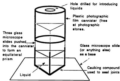
Fig 3 Hollow prism construction.
