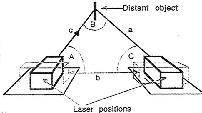
Fig 2. Laser beam range-finding.
