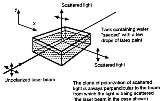
Fig 17. Polarization by scattering from a "seeded" liquid in a tank.
