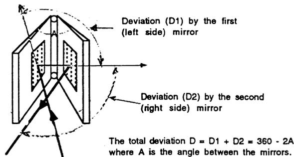
Fig 5. Beam deviations from two mirrors.
