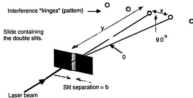
Fig 19. A double slit interference experiment.
