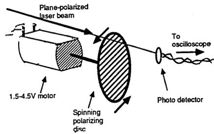
Fig 18. A system for obtaining a sinusoidal output from a photo detector.
