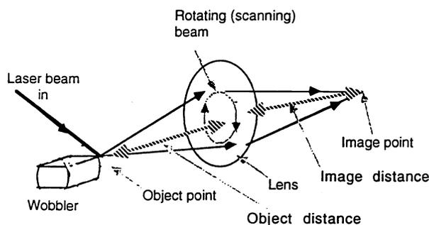
Fig 12. Measuring the focal length of a lens using the laser beam scanner.
