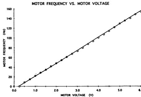
Fig 12. Speed v voltage for a Radio Shack motor.
