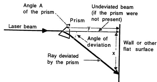
Fig 4. Minimum deviation with a prism.
