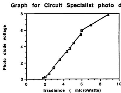
Fig 8. The voltage measured across the resistor of Fig 7 v irradiance on the photo diode.
