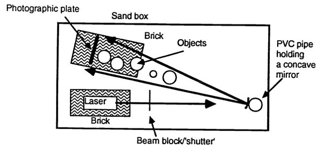
Fig 22. A plan view of a sand-box system for making transmission holograms.
