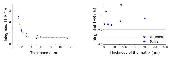
Figure 2: Evolution of the integrated THR in the UV-Vis-NIR (300-2300 nm) as a function of the thickness of the black coating (left) and the nominal thickness of the infiltrated oxide layer (right) into a ~5µm thick CNT-based composite. (AOI: 8°)
