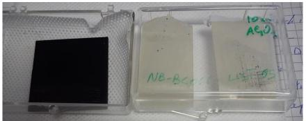
Figure 3: Adhesion/cohesion properties of coated Al sample cleaned 8 times using isopropanol and acetone soaked tissue. The black coating is reinforced in this illustration with 10nm of Al<sub>2</sub>O<sub>3</sub> Environmental tests on coated Al
