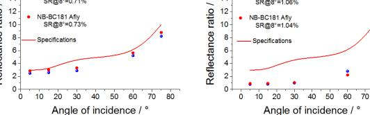
Figure 4: TIS and specular reflection measurements of the as-grown (blue) and aged (red) black coating on Al substrate. The coating process was modified by extending the hydrolysis step in the ALD process for the growth of the Al<sub>2</sub>O<sub>3</sub> reinforcement layer.
