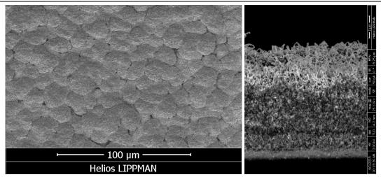
Figure 1: SEM inspection of the surface (left) and cross-section (right) of the CNT-based nanocomposite as infiltrated by 20 nm Al<sub>2</sub>O<sub>3</sub>.
