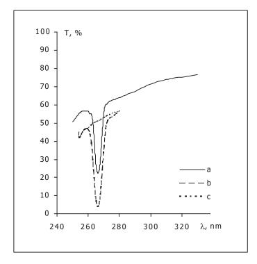
Fig.2. The transmission spectra of hologram filters in thicknesses equal to 5 (a) and 10 (b)  $\mu$ m, c-transmission of noise component of signal inside of the diffraction zone.
