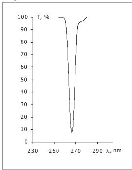
Fig.4. The differential spectrum of hologram filter in layer's thickness equal 10 μm, received from spectrum 2b in Fig.2 by differential subtraction of spectrum 2c.
