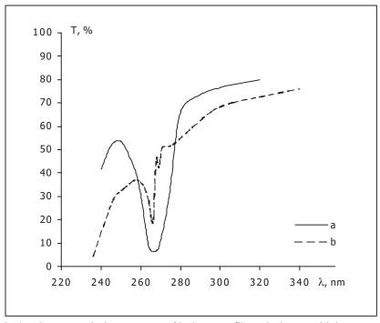
Fig.3. The transmission spectra of hologram filters in layer's thicknesses equal to 1 (a) and 23 (b) μm.
