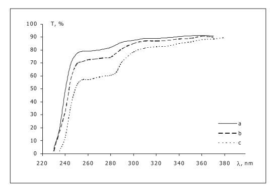
Fig.1 The transmission spectra of gelatin's layers of different thicknesses: a-5, b-10, c-23 μm
