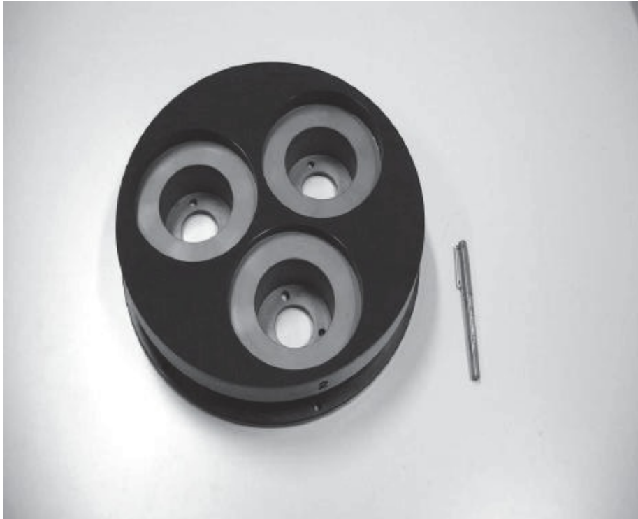
Fig. 14 : The SiC parent mirror tool. The external diameter is 330 mm.
