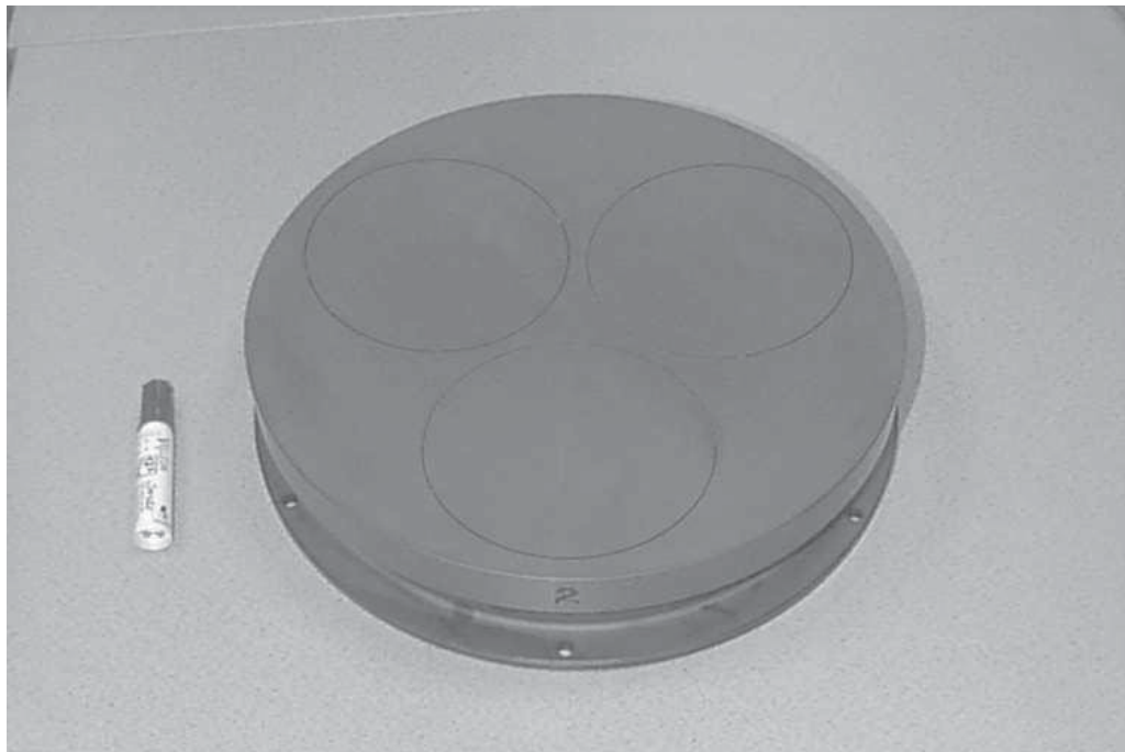
Fig. 16: The three M1 mirrors inside their parent tool ready for polishing.
