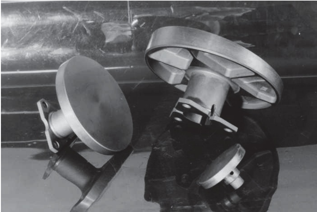
Fig. 13 : The three types of mirrors after sintering. The optical surface and mechanical fixation are parts of a single SiC element. The diameter of the larger mirror is 130 mm.
