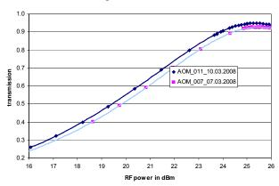
Fig. 7. Optical Transmission of the AOMs
