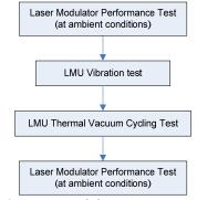
Fig. 9. Laser Modulator EM test program
