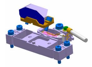
Fig. 8. Optical Path Difference Actuator
