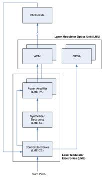
Fig. 2. Block Diagram of the Laser Modulator
