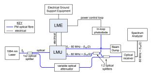
Fig. 11. Frequency stability test setup
