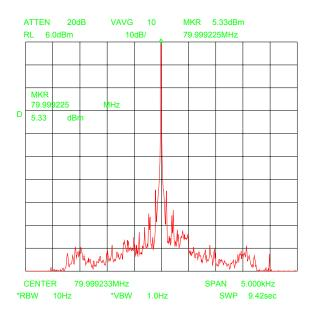
Fig. 14. Optical Spectral Purity Results with fhet = 1000 Hz for path 2 of LM EM
