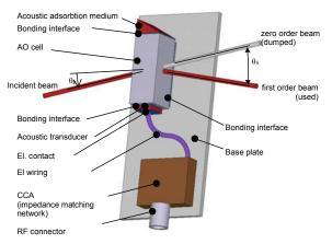
Fig. 6. Schematic Illustration of an AOM
