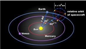
Fig. 1. Schematic of the LISA Orbit
