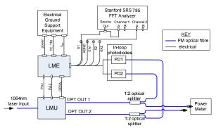
Fig. 10. LM Loop Gain test setup
