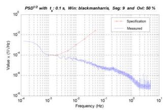
Fig. 13. MilliHertz Laser RIN of path 2.
