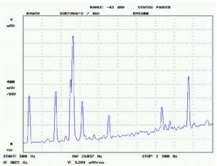
Fig. 12. Heterodyne Laser RIN of path 1 of LM EM (optical receiver DC voltage = 4.28 V)
