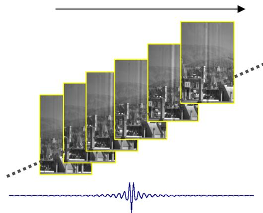
Fig. 6. The interferogram along the diagonal, the arrow is the direction of movement .
