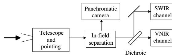
Fig. 2. Block diagram of HYC optics.
