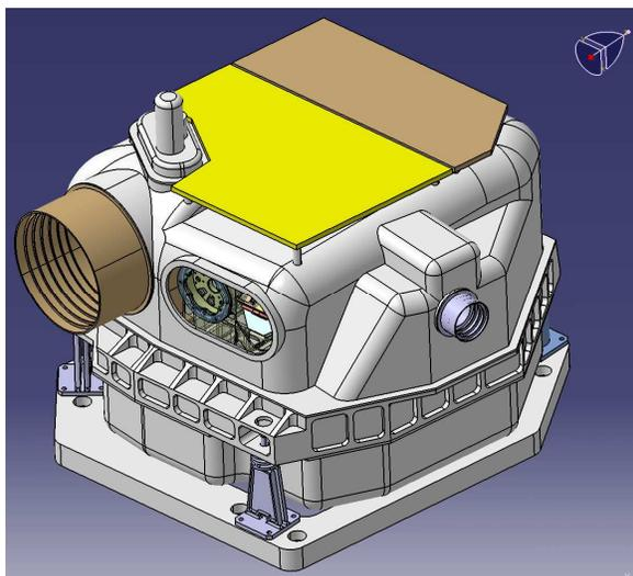
Fig. 3. Courtesy SELEX Galileo : HYP/PAN Camera Layout
