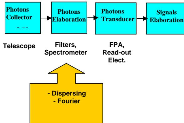
Fig. 1. Imaging Spectrometer Blocks Diagrams
