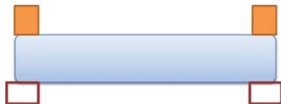
The axial mounting is less critical than the radial mounting due to the location and direction of the forces. When the spring or CTE location is opposite the support points the lens will only experience local compression forces, but no additional surface deformations will occur. Birefringence effects due to the compression stresses around the mounting points should be checked, however the affected zone will be limited.
