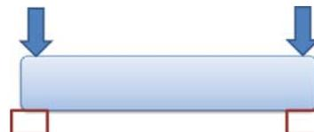
Specifically when facing high loads (e.g. during launch) gapping should be avoided thus the dimensioning of this spring can be problematic. A similar CTE compensation as for the radial support can be used for the axial support eliminating this gapping problem.
