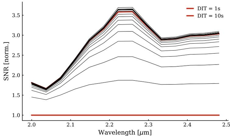
Figure 5. Signal to noise ratio estimation for different integration times, normalized by the SNR of a 1 second integration. The black lines show the SNR with an integration time between 1 and 20 seconds. The lines with 1 and 10 seconds are shown in red.
