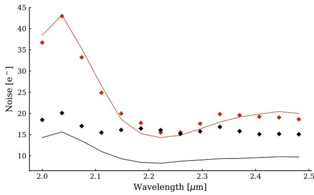
Figure 3. The dots show the measured pixel-to-pixel noise for a ten second integration (red) and a one second integration (black). The lines in the same color show the square root of the corresponding signal as an estimation of the photon noise.
