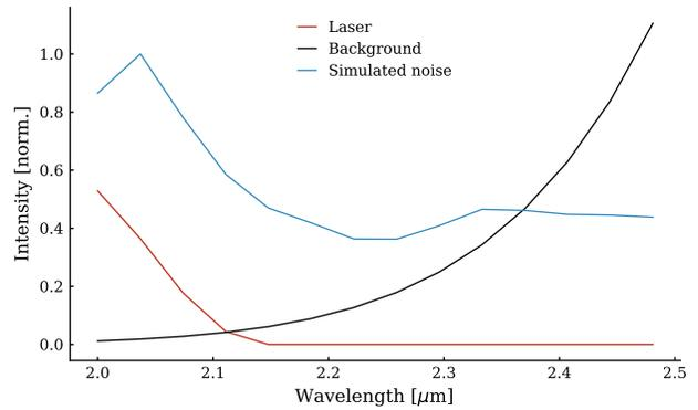
Figure 4. Estimation of the main photon noise sources of GRAVITY. The red line shows the noise from the laser backscatter, while the black line is the noise from the black body emission of the background. The typical noise at the detector is shown in blue.
