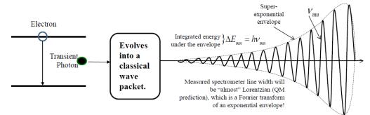
Figure.2. Hybrid photon model. At the instant of emission from atoms or molecules, the photon of energy hv is a quantum entity, which then triggers the emergence of a classical wave packet the same energy with a quasi-exponential temporal envelope and the QM-predicted carrier frequency v.
