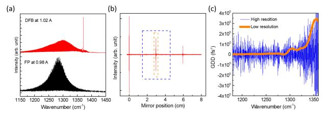
Fig. 2. (a) Measured subthreshold emission spectra for the DFB and FP devices. (b) Interferogram for the DFB spectra. The blue and orange boxes indicate the truncated mirror positions for high- and low-resolution Fourier transforms. (c) Generated high and low resolution GDD spectra. The high-resolution spectrum contains the high-frequency information with a much higher noise level than the low-resolution spectrum.
