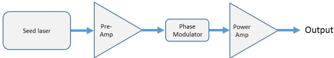
Figure 5. Schematic of CSEM laser head for LISA
