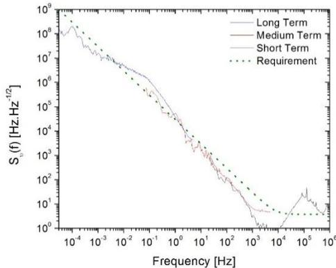
Figure 14 - LHA Frequency noise in Free-Running Mode operation.
