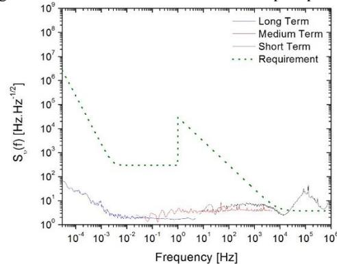
Figure 15 – LHA Frequency noise in Master Mode (locked with the ORS) operation.
