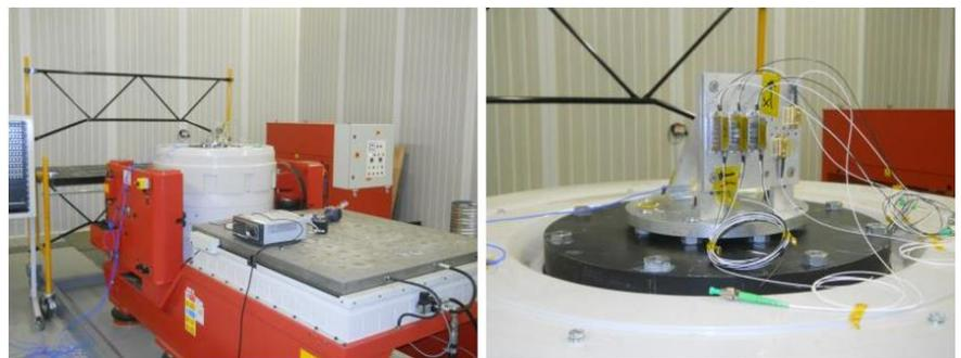
Figure 9 -Optical Switches and pump lasers under vibration testing.
