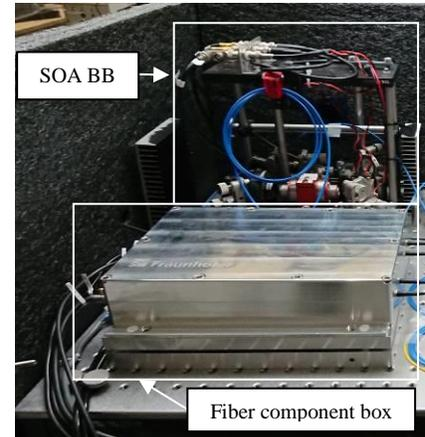
Figure 7. Fiber component box of Fiber Amplifier (front) and SOA BB setup (back).
