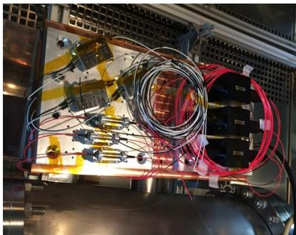
Figure 8 - Photonic devices under TVAC test.
