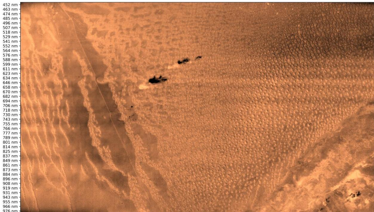
**Figure 9: Hyperspectral frame image acquired by HyperScout-1 over the invariant site Algeria-3**
