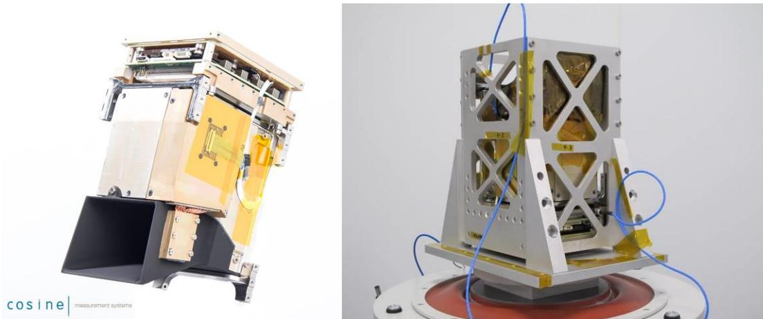
**Figure 5: The HyperScout-1 FM (left). The HyperScout-1 configured for vibration testing (right)**
