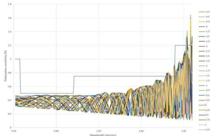
Figure 7: Polarization sensitivity (%) of the full instrument as a function of wavelength for different field angles
