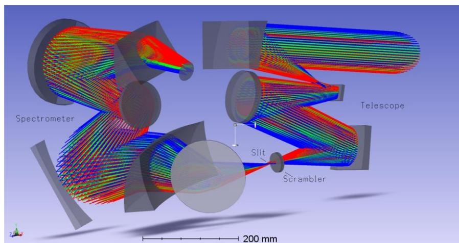
Figure 1: Full HIS optical design schematic
