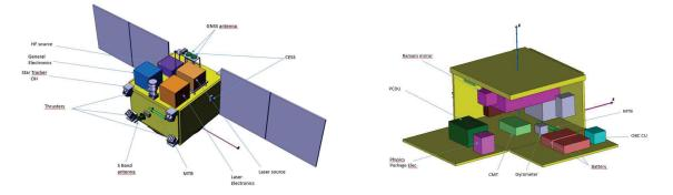
Figure 3: Preliminary design of the CARIOQA satellite platform.
