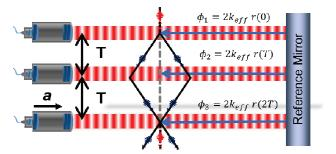
Figure 1: Scheme of a three pulses atom interferometer using Raman lasers in a retro-reflected configuration. The total interaction time is 2T. The interferometer is sensitive to the acceleration of the cold atoms with respect to the retro-reflection mirror in the direction of the Raman lasers.
