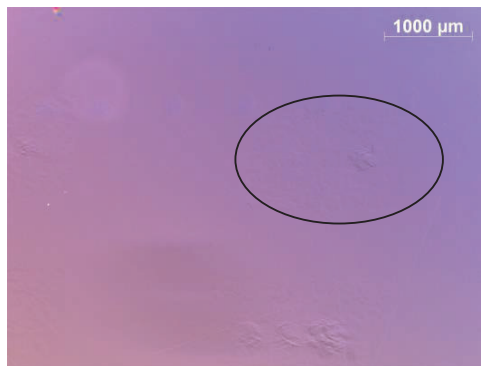
Figure 11. Soldering of a 150μm array with different parameters (4000mA, 0,5ms)
