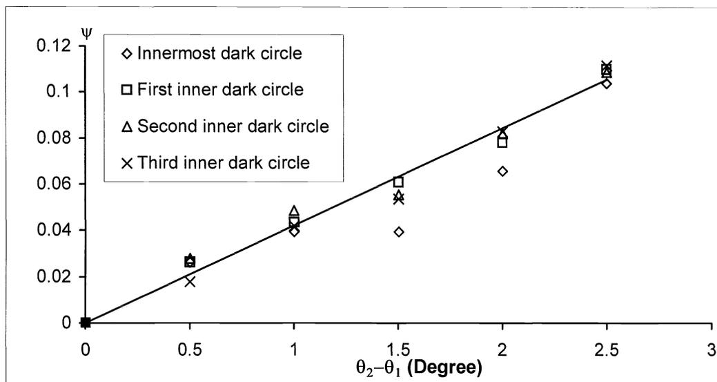
Fig. 6. Linear relationship between  $\psi$  and angular rotation of a specularly reflective surface
