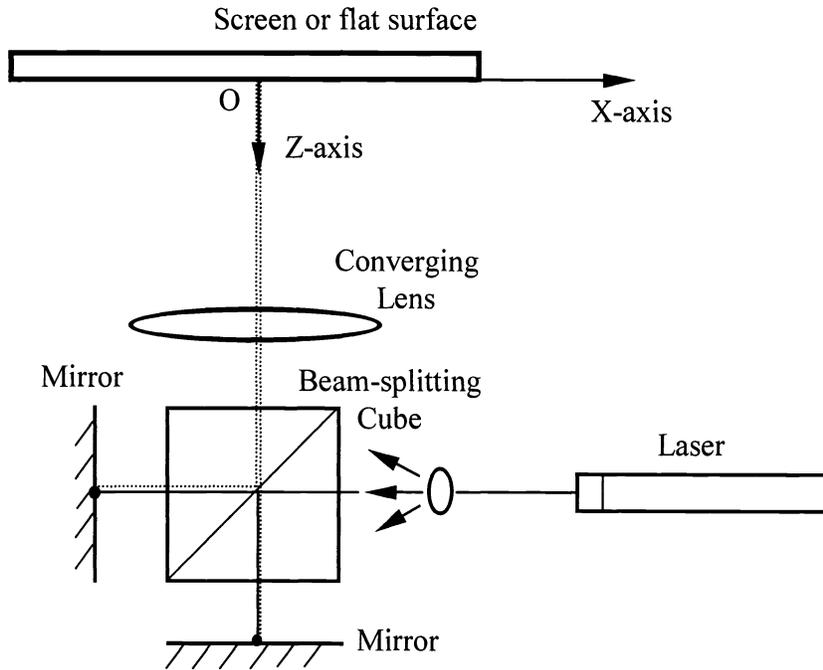
Fig. 1. Generation of optical grating using Michelson Interferometer
