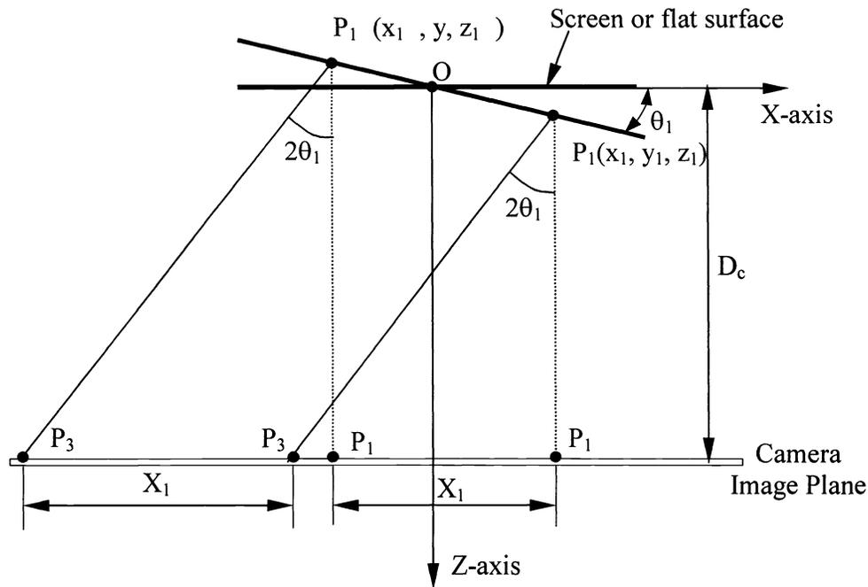
Fig. 3. Determination of the rotating angle from the distorted grating that is reflected from a mirror-like surface
