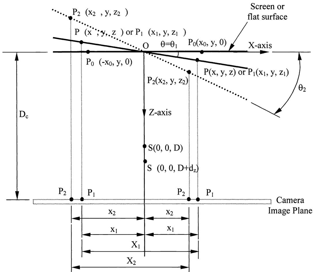
Fig. 2. Determination of the rotating angle from the distorted circular grating that appears on a diffuse/specularly reflective surface.
