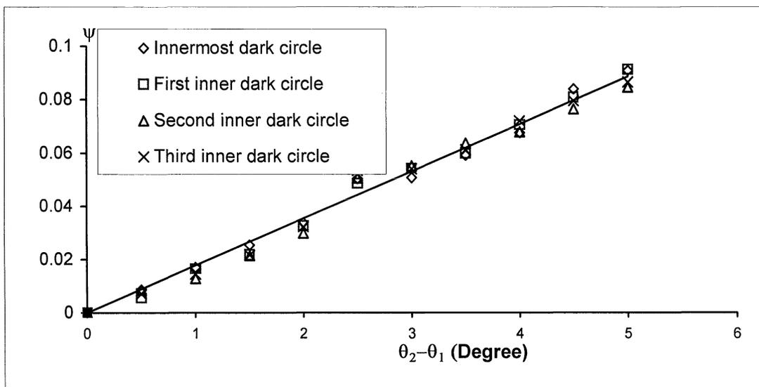
Fig. 5. Linear relationship between  $\psi$  and angular rotation of diffuse surface
