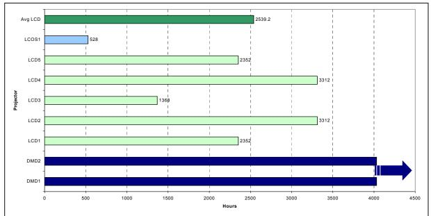
Figure 10 - Time to failure for different projector technologies.
