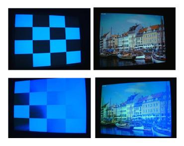
Figures 9a and 9b - Picture generated by a DMD after 3300 hours shows no degradation in image quality.
