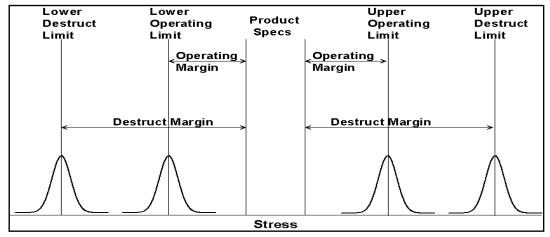
Figure 3 - Accelerated Stress Testing or Test-to-Failure Approach.
