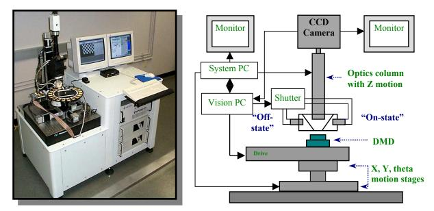
Figure 4 - DMD Test System
