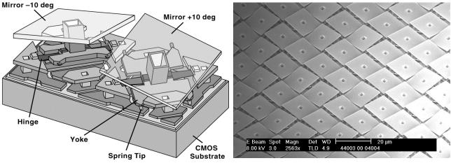
Figure 1 - Illustration of 2 landed DMD mirrors.
