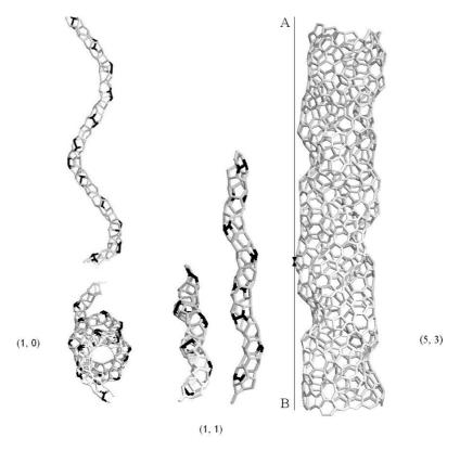
Figure 4 Curved tubular nanostructures: (1, 0) regular, helical coil; (1,0) curled tube; (5, 3) tube with mild curvature, the line AB is shown as reference for a straight object.
