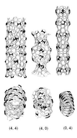
Figure 3 Tubular nanostructures generated the wrapping vectors (4, 4), (4, 0) and (0, 4), the position of the stressors is highlighted in black, the structures are shown as viewed from a direction transversal to their axes and from a view close to axial.
