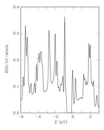
Figure 5  $\pi$ -electron density of states for the (0,4) tube calculated using a tight-binding Hamiltonian.
