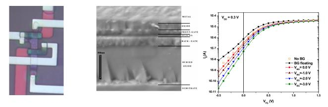
Finally, this same structure with a common floating gate between two transistors provides a method for using one transistor for programming a pass-transistor interconnection using a cross-point switch employing two programming lines. The ability to control the power and speed using the threshold voltage, achieving a non-volatile memory, and programming these properties holds great promise in
