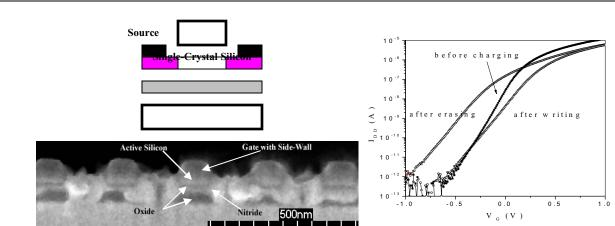
The charge is stored on defects on the back of the device structure, and the charge can be injected efficiently only at high voltages. So, these devices operate as transistors at low voltages and as memories at high voltages, and can be architecturally employed to perform both functions.
