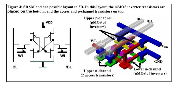
The consequence of implementing such a structure in planar CMOS technology is that a typical cell uses 80-100 squares of the lithographic feature size. And, much ingenuity in processing goes into collapsing and overlapping the interconnect structure, and cleverly eliminating design constraints in the layout of the cell. Most microprocessors, however, still utilizes half or more of the area for SRAMs that provide the on-chip cache memory hierarchy. Thus, attaining a smaller
