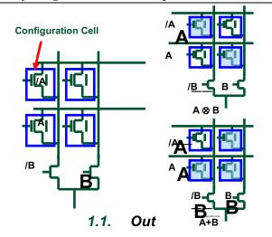
such a back-gated structure implementation where a NOR and XOR functions are implemented using the same 4 transistor circuit using the programmability achieved from the back-gate. Fig. 9 shows an example of a fabricated configurable structure using the 3D approach described.
