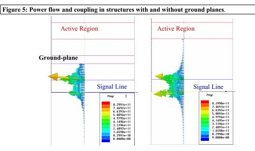
When the ground-plane is absent a substantial amount of signal energy is coupled to the active region, while the presence of a ground plane shadows and isolates the active region. The consequence of an ability to isolate such noise is that very versatile mixed-signal applications can be pursued where analog design plays as large a part as the digital design.
