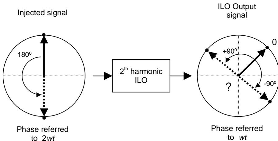
Figure 8: Phasor diagram of a 2<sup>nd</sup> harmonic ILO injected with a BPSK signal
