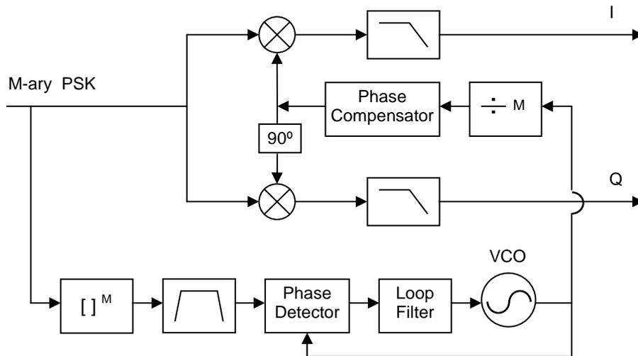
Figure 5: M-ary PSK demodulator with M powering loop carrier recovery system
