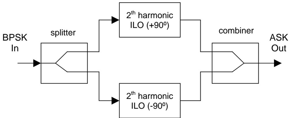
Figure 9: Block diagram of the PSK to ASK converter based on the dynamics of two ILOs.
