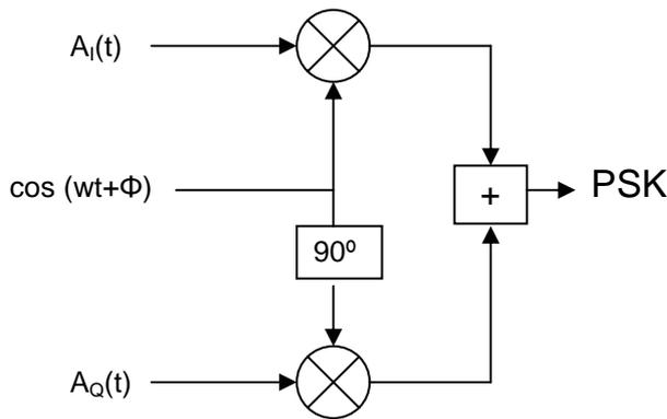
Figure 1: Schematic Block Diagram of a PSK modulator
