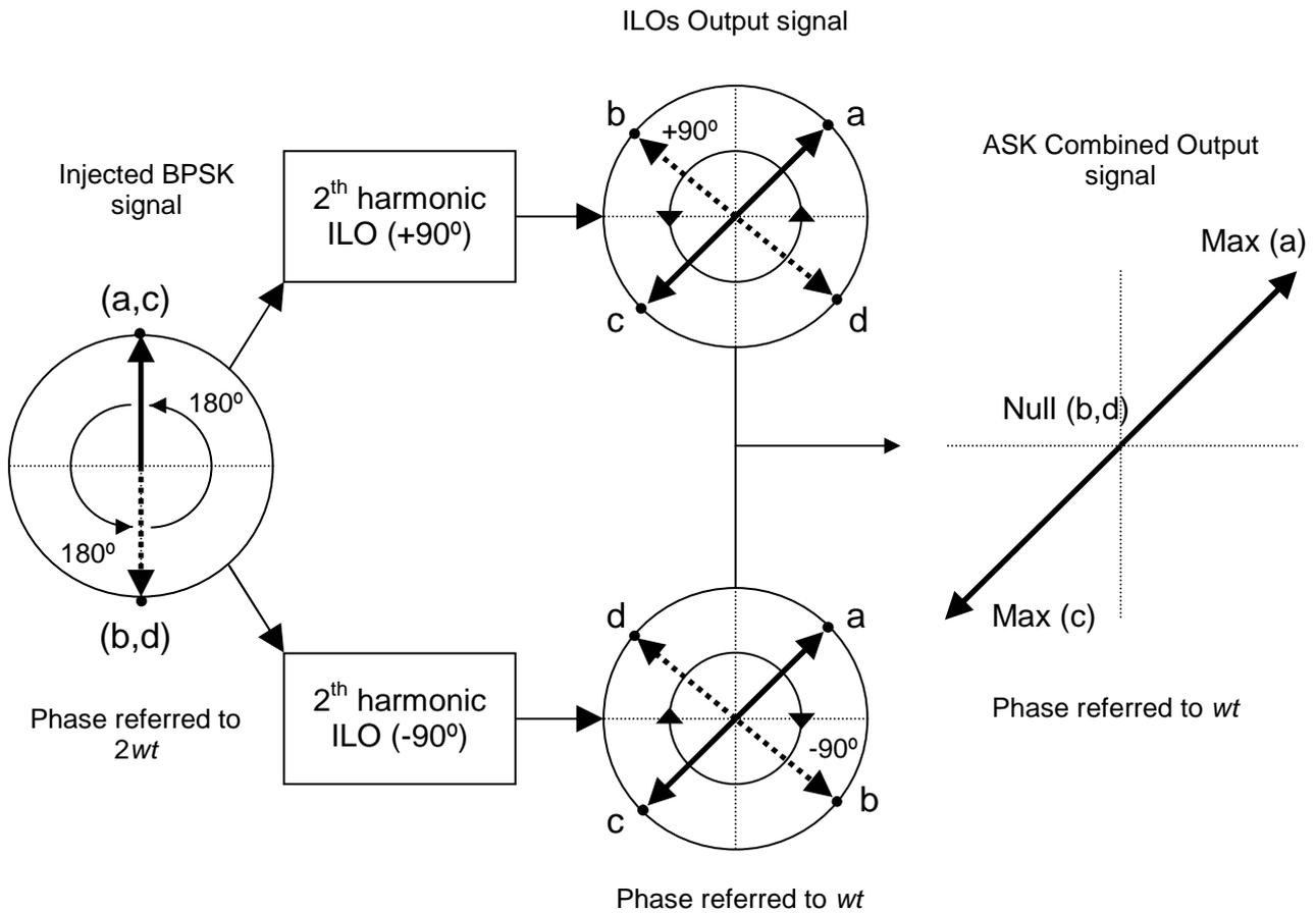
Figure 10: Phasor diagram of the BPSK to ASK conversion
