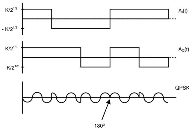
Figure 3: QPSK signal time domain waveforms
