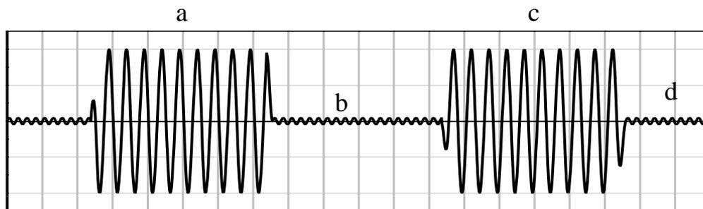
Figure 11: Time domain waveform of the ASK output
