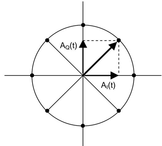
Figure 2: Constellation Diagram for a M-ary PSK signal (M=8)
