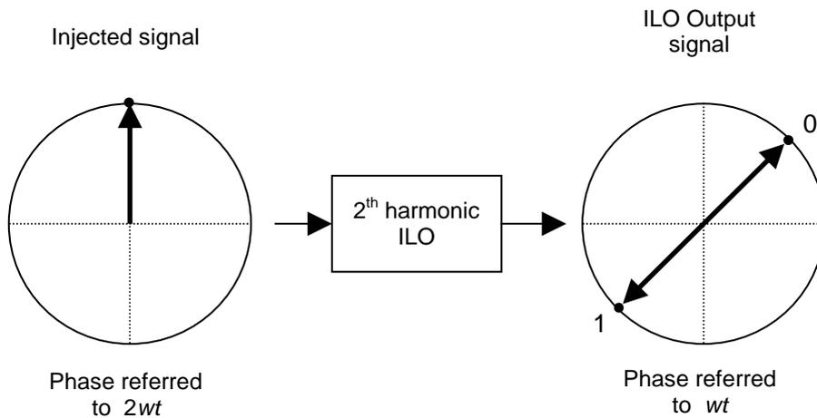
Figure 7: Phasor diagram of a 2<sup>nd</sup> harmonic ILO
