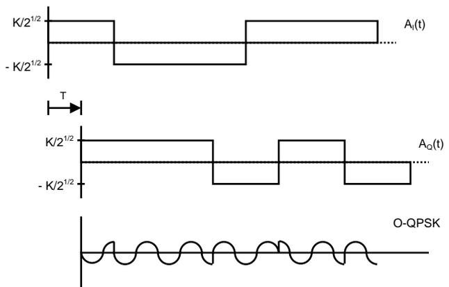
Figure 4: O-QPSK signal time domain waveforms
