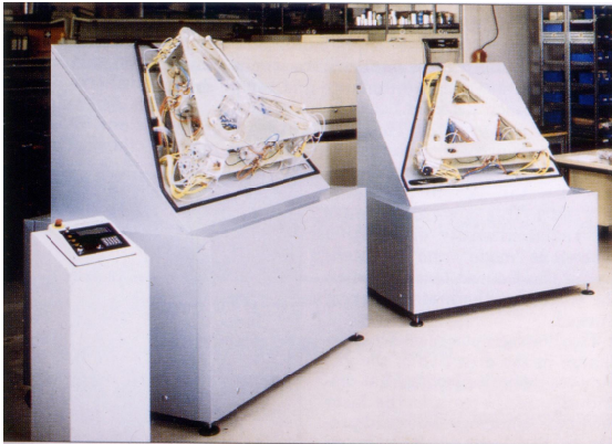
Figure 4. Fast axial flow CO 2 laser system in a triangular geometry built by Triumphf
