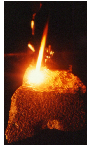
Figure 3. Effect of directing the multi-kW unfocussed CO 2 laser light on to a piece of stone
