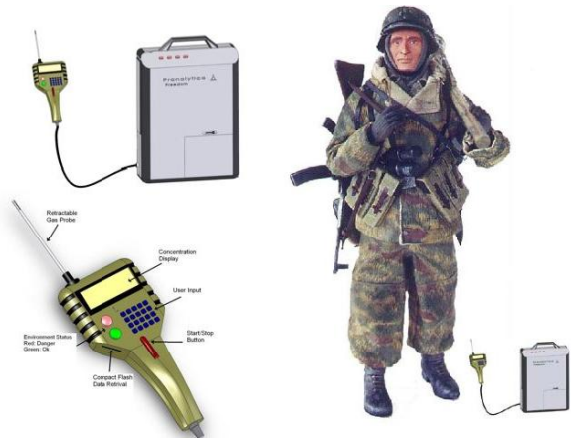
Figure 11. QCL based laser photoacoustic spectrometry based CWA sensor that will be man-portable and have very high sensitivity as well as very low false alarm rates.
