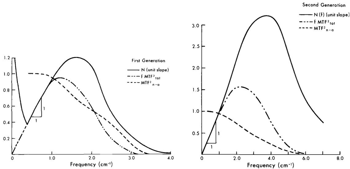
Fig. 4. Noise power spectra of (left) the EMI Mark I and (right) the EMI CT505 normalized to unit slope in low frequencies and construction for obtaining information bandwidth integral (IBWI). The ordinate scale is dimensionless except for the lower two curves for which it is in units of frequency (cycles/cm) [16].
