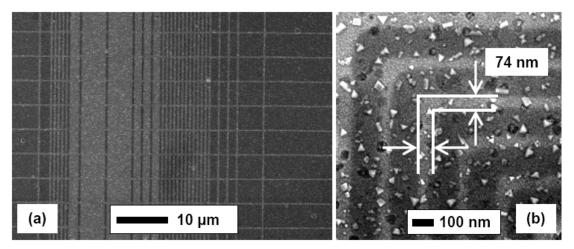
Figure 2. SEM images of YBCO thin film surfaces patterned by masked ion beam structuring. Ion irradiated regions of films appear relatively darker, non-irradiated YBCO film regions are brighter. Irradiated micro-structures (a) and nano-structures (b). Solid white lines are guides to the eye (b).
