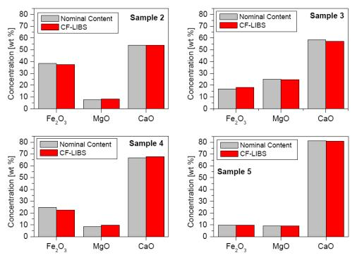
Figure 3. CF-LIBS analysis of four samples containing different amount of iron oxide, magnesium oxide, and calcium oxide. Oxide concentration as determined by CF-LIBS (red columns) and nominal concentration (grey columns).
