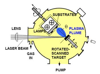
Figure 1. Schematic of experimental setup for pulsed-laser deposition of thin films in "on-axis" geometry. The distance between target and substrate is several cm, typically.
