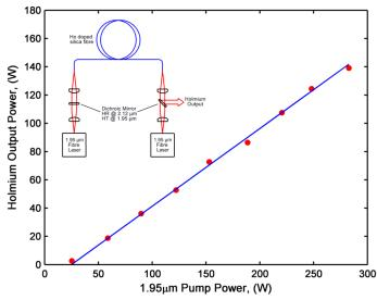
Fig. 1: Output power of holmium fibre laser vs input pump power. Inset: A schematic of the experiment.
