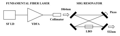
Figure 1. Experimental configuration
