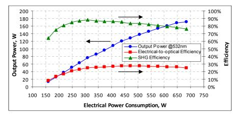
Figure 2. Output power at 532nm (blue circles), electrical-to-optical laser efficiency (red squares), and SHG efficiency (green triangles) as a function of electrical power consumption
