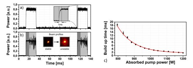
Fig. 1.: Example to illustrate a) the pulsed pump scheme and b) the detected signal above the mode instability threshold. Temporally, the amplifier showed stable fundamental-mode operation (dark gray shaded areas), but switched to unstable mode operation with a delay of some ms (light gray shaded areas).c) Mode instability build up time in dependence on the absorbed pump power.
