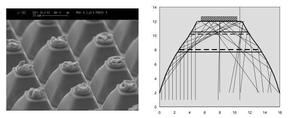
Figure 2 Deep slot structure – absorption efficiency 0.90, number of photons double-reflected into adjacent pixels (stray light) 2.3%
