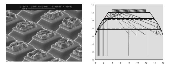
Figure 1 Standard 16 μm pitch structure – absorption efficiency 0.86, number of photons double-reflected into adjacent pixels (stray light) 3.5%
